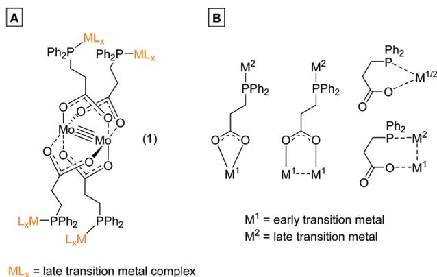
**Scheme 2** (A) Dimolybdenum(II) metalloligand (**1**) allowed the subsequent build-up of heteromultimetallic structures *via* metal coordination of the phosphine donor sites. (B) Variable coordination modes of the bifunctional ligand 3-(diphenylphosphino)propionic acid towards different metal centers. Due to the ethylene-spacer moiety between phosphine and carboxylic acid functionality the ligand can act as a flexible hemilabile ligand system.
