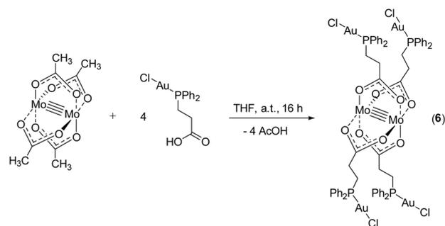
**Scheme 6** Synthesis of heteromultimetallic  $\text{Mo}_2\text{Au}_4$  compound 6 *via* carboxylate substitution from molybdenum(II) acetate. Compound 6 forms a 1D coordination polymeric structure in the solid state (scheme merely exhibits the respective monomer).
