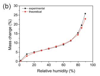
Fig. 6 Water sorption isotherms of (a) HNT (blue), sepiolite (red), CNF (green), and HNT-SEP-CNF (black) films. (b) Experimental vs. theoretical water sorption isotherms.
