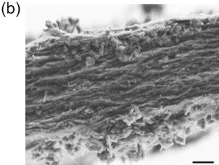
Fig. 3 SEM micrographs of (a) the surface and (b) the fracture cross-section of the 1:1:1 HNT–SEP–CNF hybrid nanopaper, respectively. The scale bars refer to 2  $\mu$ m.
