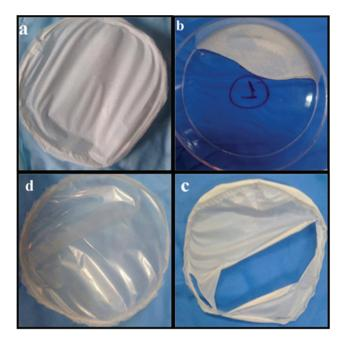
**Fig. 4** Macroscopic aspect of various hybrid films prepared by combining HNT, SEP and CNF at different weight ratios: (a) 1:1:1 HNT-SEP-CNF nanopaper, (b) 1:1 HNT-SEP, (c) 1:1 HNT-CNF, and (d) 1:1 SEP-CNF.
