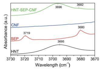
**Fig. 5** FTIR spectra of the HNT, SEP, CNF and HNT–SEP–CNF hybrid nanopaper (3730–3670  $\,\rm cm^{-1}$  range). The complete spectra are provided in Fig. S3.†
