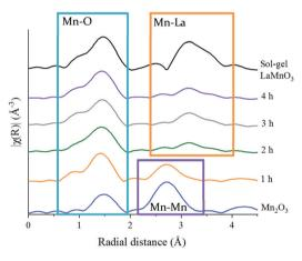
Fig. 3 Non phase-corrected Fourier transform at the Mn K-edge for LaMnO<sub>3</sub> synthesised by sol-gel and by ball milling from 1 h and 4 h compared to precursor Mn<sub>2</sub>O<sub>3</sub>.
