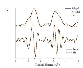
Fig. 4 Mn K-edge EXAFS data after (A) time 0 h of milling (Mn<sub>2</sub>O<sub>3</sub>) and after time (B) 1 h of milling (C) 4 h of milling compared to (D) sol-gel synthesized LaMnO<sub>3</sub> showing the magnitude and imaginary components of the  $k^2$ -weighted Fourier transform data and simulated fits.
