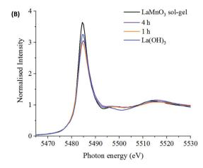
Fig. 2 XANES spectra at the (A) Mn K-edge for LaMnO<sub>3</sub> prepared by sol-gel synthesis and ball milling after 1 and 4 hours compared to Mn<sub>2</sub>O<sub>3</sub> precursor with highlighted pre-edge region and (B) La L3-edge for LaMnO3 prepared by sol-gel synthesis and ball milling after 1 and 4 hours compared to La(OH)<sub>3</sub> precursor.
