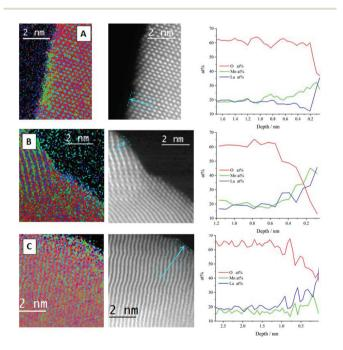
Fig. 7 STEM-EELS atomic percentage elemental mapping (left column), HAADF-STEM images with integrated profiling lines (central column) and line profiling along the arrow, for the atomic percentage of La (blue), Mn (green) and O (red) for (A) sol–gel synthesised, (B) 3 h milled and (C) 4 h milled LaMnO<sub>3</sub>.
