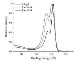
Fig. 6 XPS spectra in the O 1s region of 3, 4 h ball milled samples compared to sol-gel synthesised LaMnO<sub>3</sub>.
