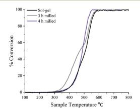
Fig. 8 Light-off curve showing the percentage of  $deN_2O$  to  $N_2$  over 3 h, 4 h ball milled and sol-gel synthesised LaMnO<sub>3</sub> using 0.5%  $N_2O/He$  at 30 mL min<sup>-1</sup> with a pre-treatment of He at 30 mL min<sup>-1</sup>.
