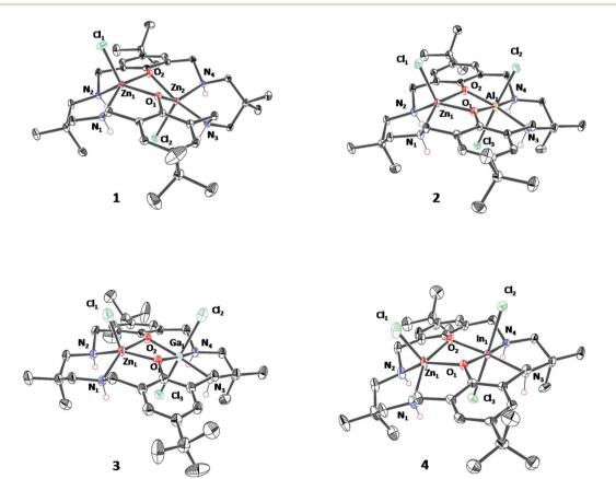
Fig. 3 ORTEP representation of the crystallographic structure of complex 1–4 and 6 obtained by single crystal X-ray diffraction. Disorder and H-atoms (excluding NH) have been omitted for clarity, with thermal ellipsoids represented at 40% probability. Selected bond lengths (Å) and angles (°) see Tables S1–S5.†
