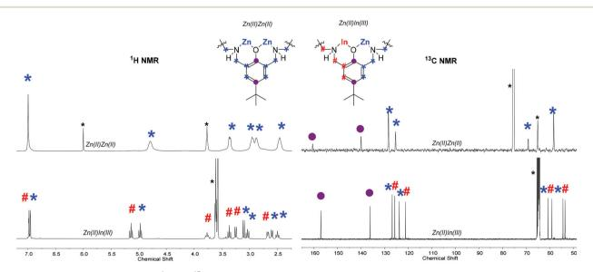
Fig. 2 Overlaid selected regions of the <sup>1</sup>H and <sup>13</sup>C NMR spectra of di-zinc complex (1) and heterodinuclear Zn(II)In(III) complex (4). Note the full spectra and assignment is available in the ESI (Fig. S1, S2, S12 and S15†). \*Residual TCE and THF.
