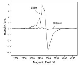
Fig. 4 EPR spectra of the calcined and spent V/SBA-15.
