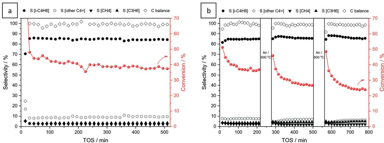
Fig. 5 Catalytic performance of V/SBA-15 in the non-oxidative dehydrogenation of isobutane: conversion (right axis), carbon balance (left axis) and selectivity to different products ( $S[-]$ , left axis) at 550 °C and  $WHSV = 240 \text{ mL min}^{-1} \text{ g}_{\text{cat}}^{-1}$  for 520 minutes of experiment (a) and by applying cycles of reaction-regeneration\* of 4–1 hours (b). \*Regeneration conditions: 50  $\text{mL min}^{-1}$  of air at 600 °C for 1 hour.
