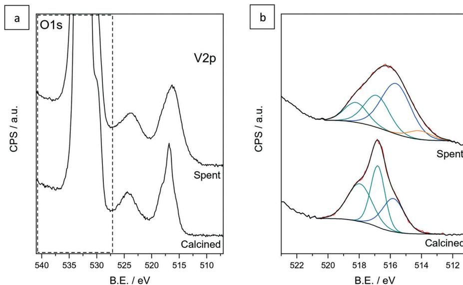
**Fig. 3** XPS spectra of the calcined and spent V/SBA-15 samples in the O1s + V2p region (a) and detailed/deconvoluted V2p<sub>3/2</sub> spectra (b). V<sup>5+</sup>, V<sup>4+</sup> and V<sup>3+</sup> components are marked in green, blue and orange, respectively. The red line corresponds to the envelope of the fitted peaks.
