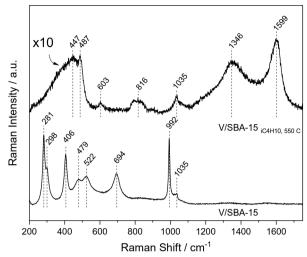
Fig. 2 Raman spectra of calcined and spent V/SBA-15 catalysts (for clarity, the spectra are offset).
