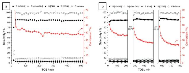
Fig. 5 Catalytic performance of V/SBA-15 in the non-oxidative dehydrogenation of isobutane: conversion (right axis), carbon balance (left axis) and selectivity to different products (S[-], left axis) at 550 °C and WHSV = 240 mL min<sup>-1</sup> g<sub>cat</sub> <sup>-1</sup> for 520 minutes of experiment (a) and by applying cycles of reaction-regeneration\* of 4-1 hours (b). \*Regeneration conditions: 50 mL min<sup>-1</sup> of air at 600 °C for 1 hour.
