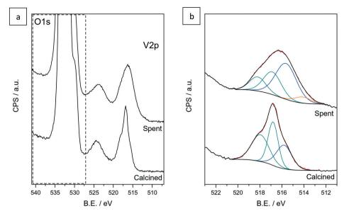
Fig. 3 XPS spectra of the calcined and spent V/SBA-15 samples in the O1s + V2p region (a) and detailed/deconvoluted V2p<sub>3/2</sub> spectra (b).  $V^{5+}$ ,  $V^{4+}$ and V3+ components are marked in green, blue and orange, respectively. The red line corresponds to the envelope of the fitted peaks.
