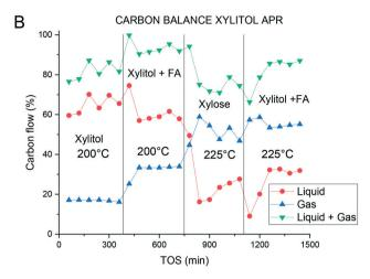
Fig. 5 Carbon balance in A) xylose and B) xylitol APR.
