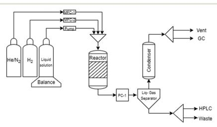
Fig. 1 Experimental set-up for aqueous phase reforming
