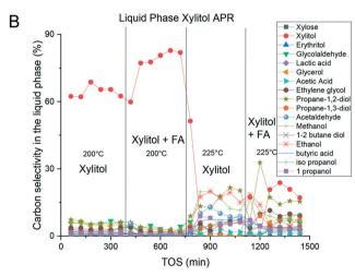
Fig. 8 Distribution of the liquid phase products in the APR of A) xylose and B) xylitol.
