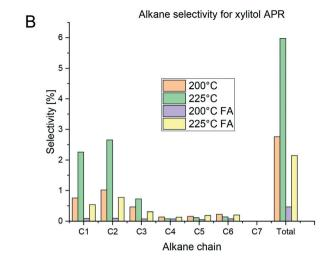
Fig. 7 Alkane selectivity in APR of A) xylose and B) xylitol.
