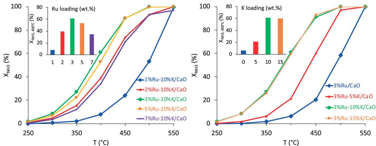
Fig. 3 Ammonia conversion versus temperature of Ru-K/CaO catalysts; effect of Ru and K loadings.  $P = 1$  atm;  $T = 250$ – $550$  °C;  $\text{NH}_3$  flow rate  $30$   $\text{N ml min}^{-1}$ ;  $W_{\text{cat}} = 200$  mg;  $\text{WHSV} = 9000$   $\text{mL g}^{-1} \text{h}^{-1}$ .
