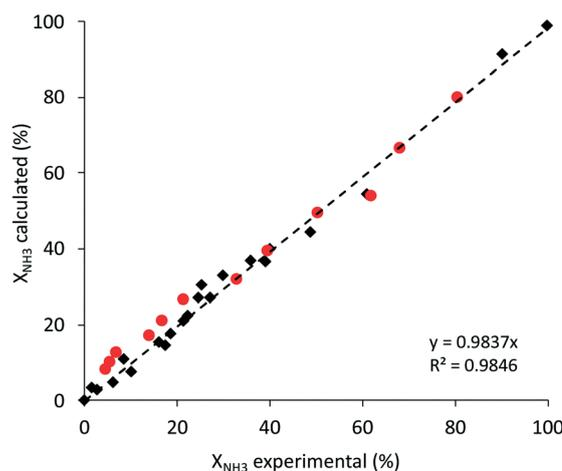
**Fig. 6** Experimental vs. modeled ammonia conversion using the proposed power-law model (eqn (2)) for ammonia decomposition over the 3%Ru10%K/CaO catalyst. Red: ammonia conversion at high pressure. Black: conversion at atmospheric pressure.
