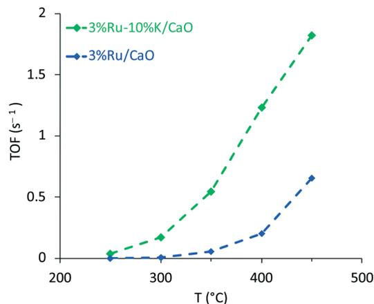
**Fig. 5** Calculated turnover frequencies (TOFs) for K-promoted and unpromoted Ru/CaO catalysts.  $P = 1$  atm;  $T = 150$ – $500$  °C;  $\text{NH}_3$  flow rate  $30 \text{ ml min}^{-1}$ ;  $\text{WHSV} = 9000 \text{ mL h}^{-1} \text{ g}^{-1}$ .
