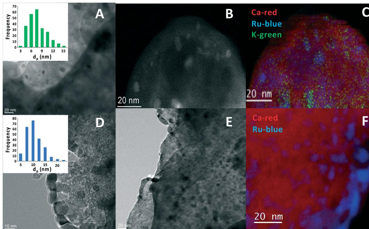
**Fig. 2** Representative images for 3%Ru10%K/CaO (A–C) and 3%Ru/CaO (D–F) after activation under hydrogen at 525 °C for 3 h, high-angle annular dark-field scanning transmission electron microscopy (HAADF-STEM) and energy-dispersive X-ray spectroscopy (EDX) images. Elemental mapping images for Ru (blue), calcium (red), and potassium (green).
