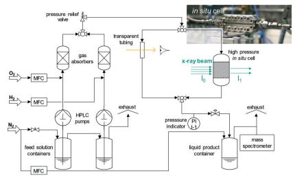
Fig. 1 Scheme of the experimental setup for operando studies of the direct H<sub>2</sub>O<sub>2</sub> synthesis and a photo of the reactor (in situ cell, top right).
