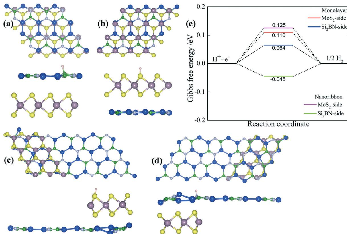
**Fig. 6** (a–d) Top and side views of monolayer and ribbon MoS<sub>2</sub>/Si<sub>2</sub>BN with a hydrogen atom adsorbed at the most favorable site on both sides. (e) Calculated Gibbs free energy profile for the hydrogen evolution reaction (HER) on both sides of monolayer MoS<sub>2</sub>/Si<sub>2</sub>BN and ribbon MoS<sub>2</sub>/Si<sub>2</sub>BN.
