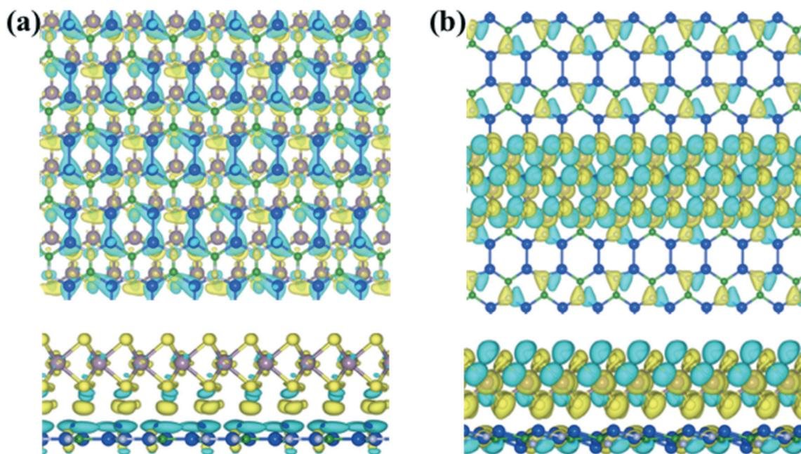
**Fig. 3** Top view (upper panel) and side view (lower panel) of the electron density difference plots for the (a) mMoS<sub>2</sub>/Si<sub>2</sub>BN and (b) rMoS<sub>2</sub>/Si<sub>2</sub>BN heterostructures. The iso-value is set as  $10^{-3} \text{ e } \text{Å}^{-3}$ . The cyan and yellow colors represent the charge depletion and accumulation in space, respectively.
