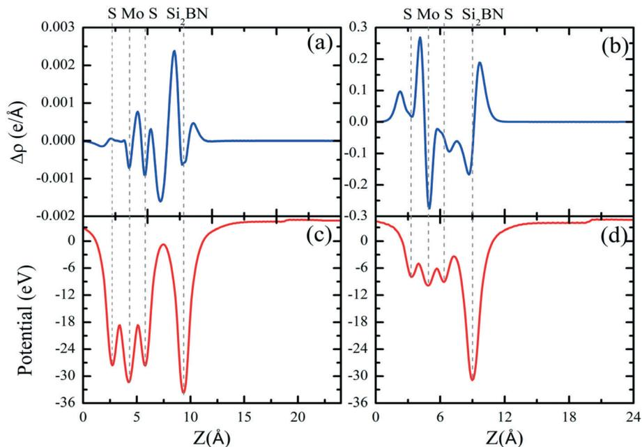
Fig. 4 Planar-averaged electron density differences  $\Delta\rho(z)$  for the (a) mMoS<sub>2</sub>/Si<sub>2</sub>BN and (b) rMoS<sub>2</sub>/Si<sub>2</sub>BN heterostructures. The electrostatic potentials for the (c) mMoS<sub>2</sub>/Si<sub>2</sub>BN and (d) rMoS<sub>2</sub>/Si<sub>2</sub>BN heterostructures.
