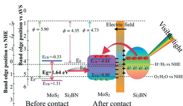
Fig. 7 A schematic diagram of the band configuration and the charge separation at the interface of MoS<sub>2</sub>/Si<sub>2</sub>BN under visible-light irradiation.
