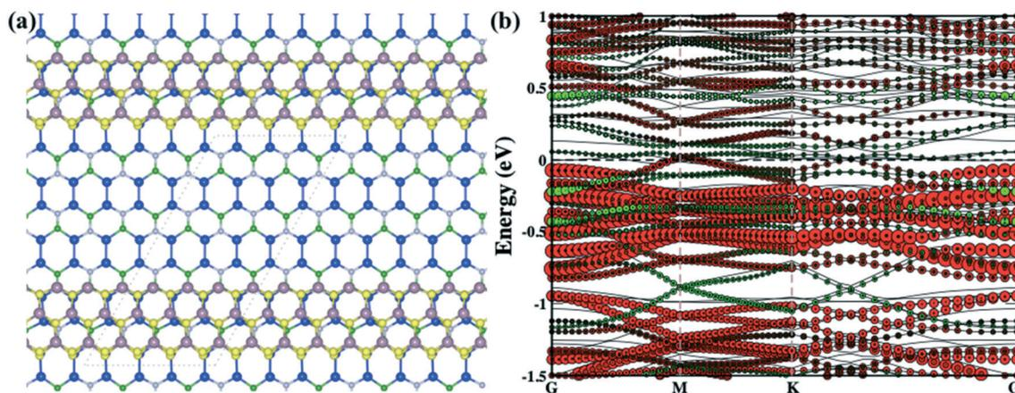
Fig. 2 The optimized  $\text{rMoS}_2/\text{Si}_2\text{BN}$  heterostructure (a) and the corresponding band structure (b) (green and red colors represent the electronic band lines of  $\text{Si}_2\text{BN}$  and  $\text{MoS}_2$ , respectively).
