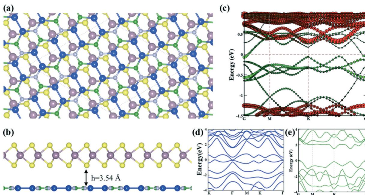
Fig. 1 The optimized mMoS<sub>2</sub>/Si<sub>2</sub>BN heterostructure viewed from the (a) top and (b) side and the (c) corresponding band structure (green and red colors represent the electronic band lines of Si<sub>2</sub>BN and MoS<sub>2</sub>, respectively). The electronic band structures of pristine (d) Si<sub>2</sub>BN and (e) MoS<sub>2</sub> monolayers.
