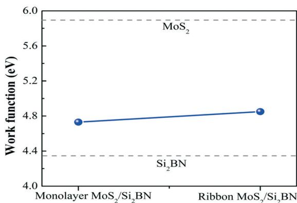
Fig. 5 Work functions of mMoS<sub>2</sub>/Si<sub>2</sub>BN and rMoS<sub>2</sub>/Si<sub>2</sub>BN. The dotted lines for pristine MoS<sub>2</sub> and Si<sub>2</sub>BN are also shown for comparison.
