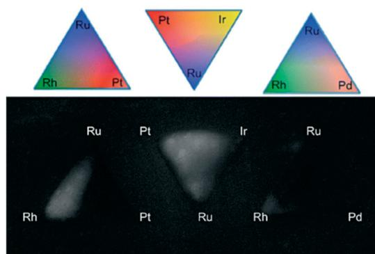
Fig. 9 Screening of gradient mixtures of platinum group metals (Pt, Pd, Ru, Rh and Ir) deposited using inkjet printing. Reprinted with permission from *ACS Comb. Sci.*, **15**, 82–89 (2013). Copyright 2013 American Chemical Society.<sup>69</sup>
