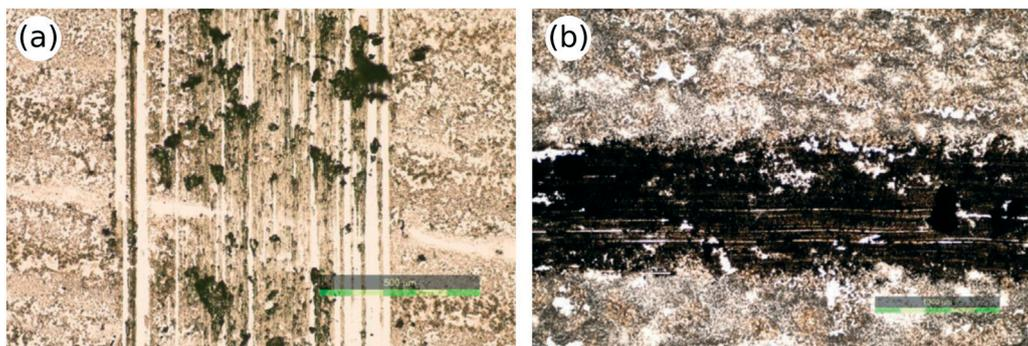
Fig. 7 TiO<sub>2</sub> thin-films after pencil hardness test: HB pencil hardness test (a) and B pencil hardness test (b). Reprinted from *Appl. Catal., B.*, vol. 138–139, M. Černá, M. Veselý, P. Dzik, C. Guillard, E. Puzenat, M. Lepičová, Fabrication, characterization and photocatalytic activity of TiO<sub>2</sub> layers prepared by inkjet printing of stabilized nanocrystalline suspensions, pp. 84–94, Copyright (2013), with permission from Elsevier.<sup>74</sup>
