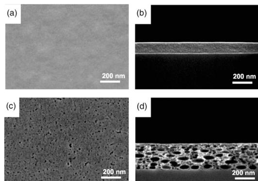
**Fig. 4** Top view and cross-sectional SEM images of as-printed  $\text{SnCl}_4$  precursor film before (a and b) and after annealing (c and d) in air at 500 °C for 15 min. Reprinted with permission from *Electrochem. Solid-State Lett.*, 10, K51–K54 (2007). Copyright 2007, The Electrochemical Society.<sup>104</sup>
