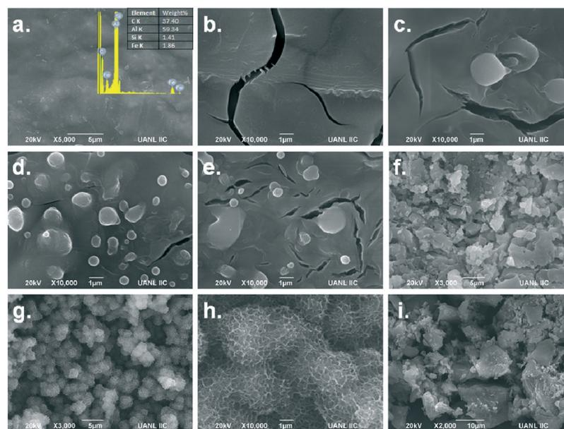
**Fig. 5** SEM images of  $\text{AlMgX}$  layers:  $X = 0$  (a), 1 (b), 3 (c), 5 (d), 10 (e), 20 (f), 30 (g and h) and 40 (i). Reprinted with permission from *Top. Catal.*, 15 (2018). Copyright 2018 Springer Nature.<sup>90</sup>
