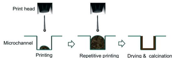
Fig. 18 Schematic illustration of deposition of nanoparticle-based inks in microchannels: inkjet printing, drying and calcination process. Reprinted from *Appl. Catal., A*, vol. 467, S. Lee, T. Boeltken, A. K. Mogalicherla, U. Gerhards, P. Pfeifer, R. Dittmeyer, Inkjet printing of porous nanoparticle-based catalyst layers in microchannel reactors, pp. 69–75, Copyright (2013), with permission from Elsevier.<sup>99</sup>
