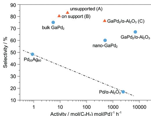
Fig. 17 Activity and selectivity of different printing approach A–C and comparison with the literature<sup>152</sup> for  $\text{Pd}_{20}\text{Ag}_{80}$ ,  $\text{Pd}/\alpha\text{-Al}_2\text{O}_3$  and  $\text{GaPd}_2$  bulk as well as nanoparticle samples. Adapted from ref. 97 with permission from John Wiley and Sons.
