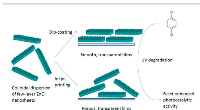
Fig. 6 Schematic illustration of deposition of active ZnO nanosheets via dip-coating and inkjet printing for UV degradation reaction. Reprinted with permission from *Langmuir*. **30**, 380–386 (2014). Copyright 2014 American Chemical Society.<sup>92</sup>
