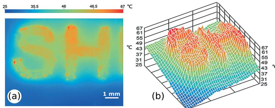
Fig. 11 The infrared thermographic image (a) and 3D temperature profile (b) of inkjet-printed Pt catalyst pattern “SH” during the methanol catalytic combustion. Reproduced from *J. Power Sources*, vol. 271, X. Luo, Z. Zeng, X. Wang, J. Xiao, Z. Gan, H. Wu, Z. Hu, Preparing two-dimensional nano-catalytic combustion patterns using direct inkjet printing, pp. 174–179, Copyright (2014), with permission from Elsevier.<sup>141</sup>
