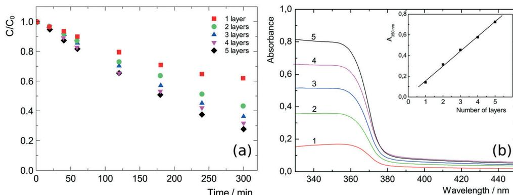
**Fig. 15** (a) Photodegradation of 4-chlorophenol on printed ZnO films: 1 to 5 layers. Reproduced with permission from *Langmuir*, **30**, 380–386 (2014). Copyright 2014 American Chemical Society. (b) UV/vis absorption spectra of 1 to 5 printed layers of the ZnO nanosheets; inset: absorbance at 350 nm with increasing number of the ZnO layers. Reprinted with permission from the supplementary information of the same reference.<sup>92</sup>
