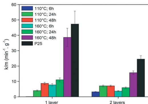
Fig. 14 Rate of 2,6-dichloroindophenol decomposition per gram of TiO<sub>2</sub> photocatalysts synthesized at different conditions. Reprinted from *Appl. Catal., B.*, vol. 138–139, M. Černá, M. Veselý, P. Dzik, C. Guillard, E. Puzenat, M. Lepičová, Fabrication, characterization and photocatalytic activity of TiO<sub>2</sub> layers prepared by inkjet printing of stabilized nanocrystalline suspensions, pp. 84–94, Copyright (2013), with permission from Elsevier.<sup>74</sup>
