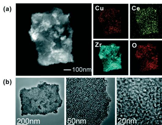
**Fig. 16** (a) STEM image and elemental mapping of the mixed metal components. (b) TEM images of the mesoporous  $\text{Cu-Ce-Zr-O}$  structure at different magnifications. Reprinted from ref. 96 with permission from the Royal Society of Chemistry.
