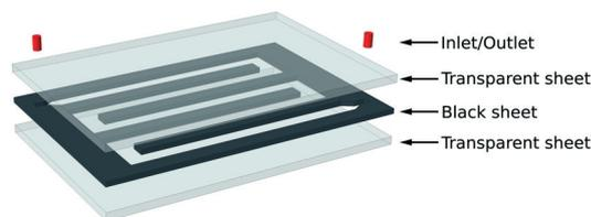
**Fig. 20** Polypropylene microreactor manufactured by laser welding with specified parts for photocatalytic studies. Available in “TiO<sub>2</sub> nanofilms on polymeric substrates for the photocatalytic degradation of methylene blue” under a Creative Commons Attribution 4.0 International Licence. Full terms at <https://creativecommons.org/licenses/by/4.0>.<sup>46</sup>
