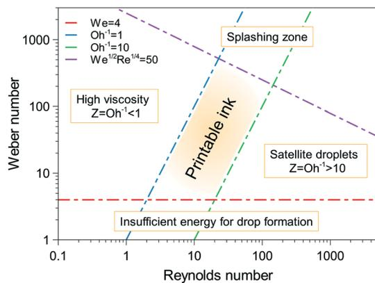
Fig. 2 Ink printability region-based the Reynolds and Weber numbers. Reproduced from *J. Eur. Ceram. Soc.*, vol. 31, B. Derby, Inkjet printing ceramics: from drops to solid, pp. 2543–2550, Copyright (2011), with permission from Elsevier.<sup>63</sup>
