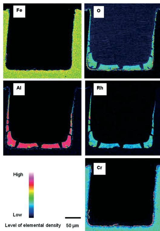
Fig. 19 Cross sectional elemental mapping images of  $\text{Rh}/\text{Al}_2\text{O}_3$  layers printed in a rectangular microchannel. Reprinted from *Appl. Catal., A*, vol. 467, S. Lee, T. Boeltken, A. K. Mogalicherla, U. Gerhards, P. Pfeifer, R. Dittmeyer, Inkjet printing of porous nanoparticle-based catalyst layers in microchannel reactors, pp. 69–75, Copyright (2013), with permission from Elsevier.<sup>99</sup>
