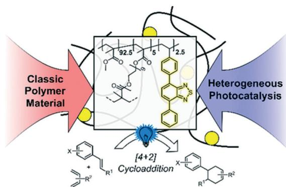
**Scheme 1** Illustration of the design concept of the PMMA-based photocatalyst copolymer and its application in the photocatalytic [4 + 2] cycloaddition.
