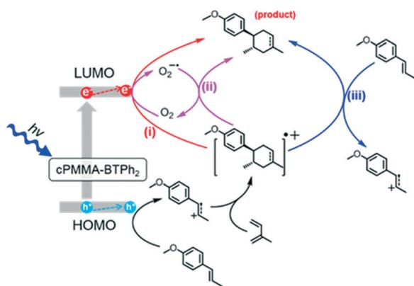
Fig. 2 Proposed reaction mechanism of the photocatalytic [4 + 2] cycloaddition using cPMMA-BTPH<sub>2</sub> as the photocatalyst.
