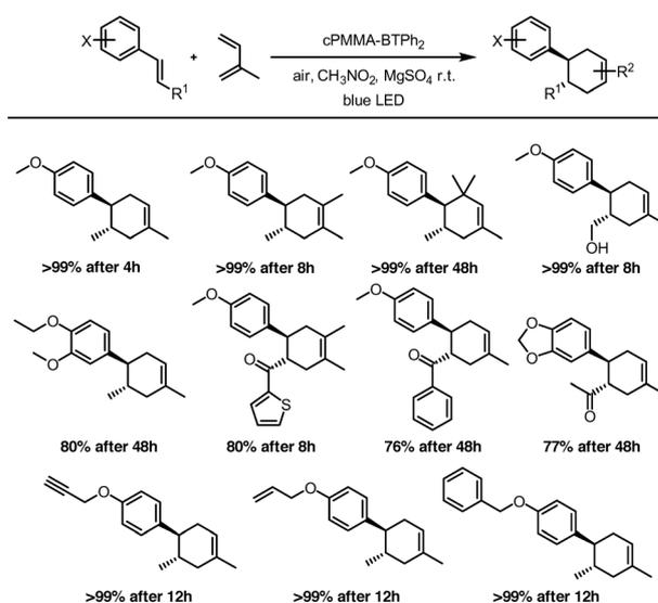
Fig. 4 Scope of the photocatalytic Diels–Alder reaction using cPMMA-BTPH<sub>2</sub> as the photocatalyst. The reactions were irradiated with a blue LED lamp (460 nm,  $0.16$  W cm<sup>-2</sup>).
