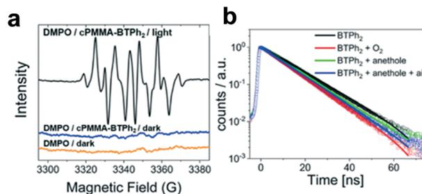
Fig. 3 (a) EPR spectra of DMPO–O<sub>2</sub><sup>•-</sup> adducts with cPMMA-BTPH<sub>2</sub> as the photocatalyst in darkness and under blue light irradiation ( $\lambda = 460$  nm,  $1.2$  W cm<sup>-2</sup>). (b) Time-resolved photoluminescence spectra of BTPH<sub>2</sub> under N<sub>2</sub> (black), under O<sub>2</sub> (red), and with *trans*-anethole under N<sub>2</sub> (green) and in air (blue) with  $20$  mg mL<sup>-1</sup> of BTPH<sub>2</sub> and  $2$  mM *trans*-anethole in acetonitrile.
