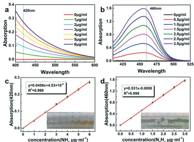
Fig. 5 (a) UV-vis curves of Nessler's reagent tests with  $\text{NH}_4^+$  ions. (b) UV-vis curves of Watt and Chrisp method tests with hydrazine. (c) Calibration curve used for the estimation of  $\text{NH}_3$ . (d) Calibration curve used for the estimation of hydrazine.
