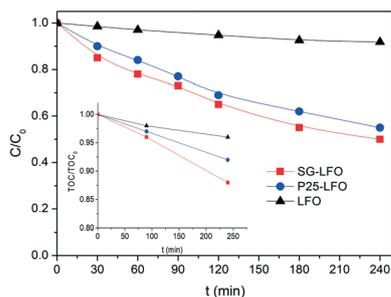
**Fig. 8** Time-evolution of both the  $C/C_0$  and  $TOC/TOC_0$  relative concentrations during the pure photocatalytic degradation of 4-CP over the pristine and the Ti-substituted  $LaFeO_3$  catalysts. Conditions:  $[4-CP]_0 = 25 \text{ mg L}^{-1}$ ;  $T = 25 \text{ }^\circ\text{C}$ ;  $[cat] = 0.5 \text{ g L}^{-1}$ ; UV-A irradiance of  $60 \text{ W m}^{-2}$ .
