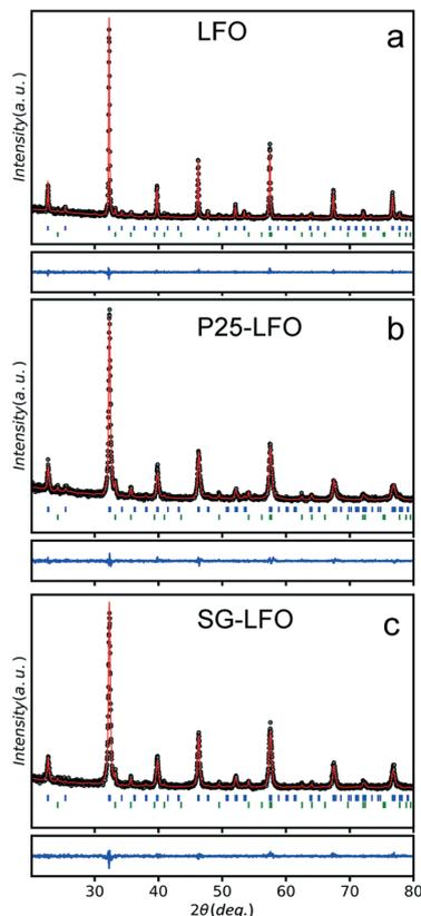
**Fig. 1** Observed (black), calculated (red full line), and difference (blue full line) X-ray powder diffraction patterns of (a) LFO, (b) P25-LFO and (c) SG-LFO catalysts recorded on a D8 diffractometer ( $\lambda = 1.54056 \text{ \AA}$ ). The positions of the Bragg reflections are represented by vertical bars, in blue for the reflections indexed in the  $Pbnm$  orthorhombic unit cell of  $\text{LaFeO}_3$  and in green for those of the  $\alpha\text{-Fe}_2\text{O}_3$  extra phase.
