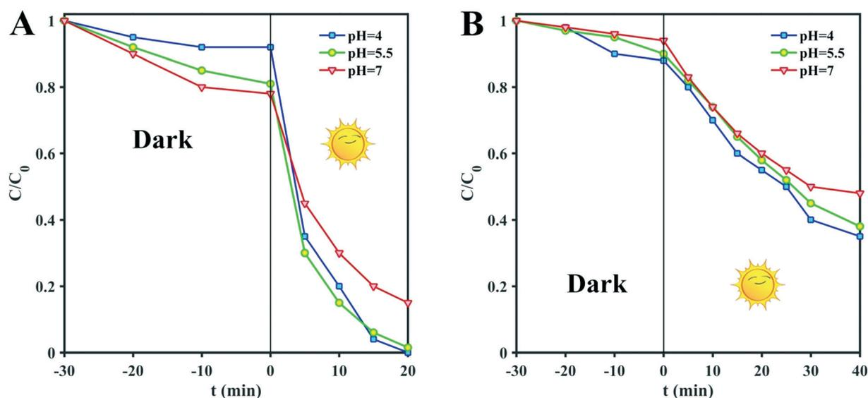
Fig. 3 Percentages of MB remaining in aqueous solutions over time in the presence of H<sub>2</sub>O<sub>2</sub>/photocatalyst/sunlight at different pH values. Part A corresponds to D<sub>1</sub> and part B corresponds to D<sub>2</sub>; 100 mL of 150 ppm MB was used in each experiment.
