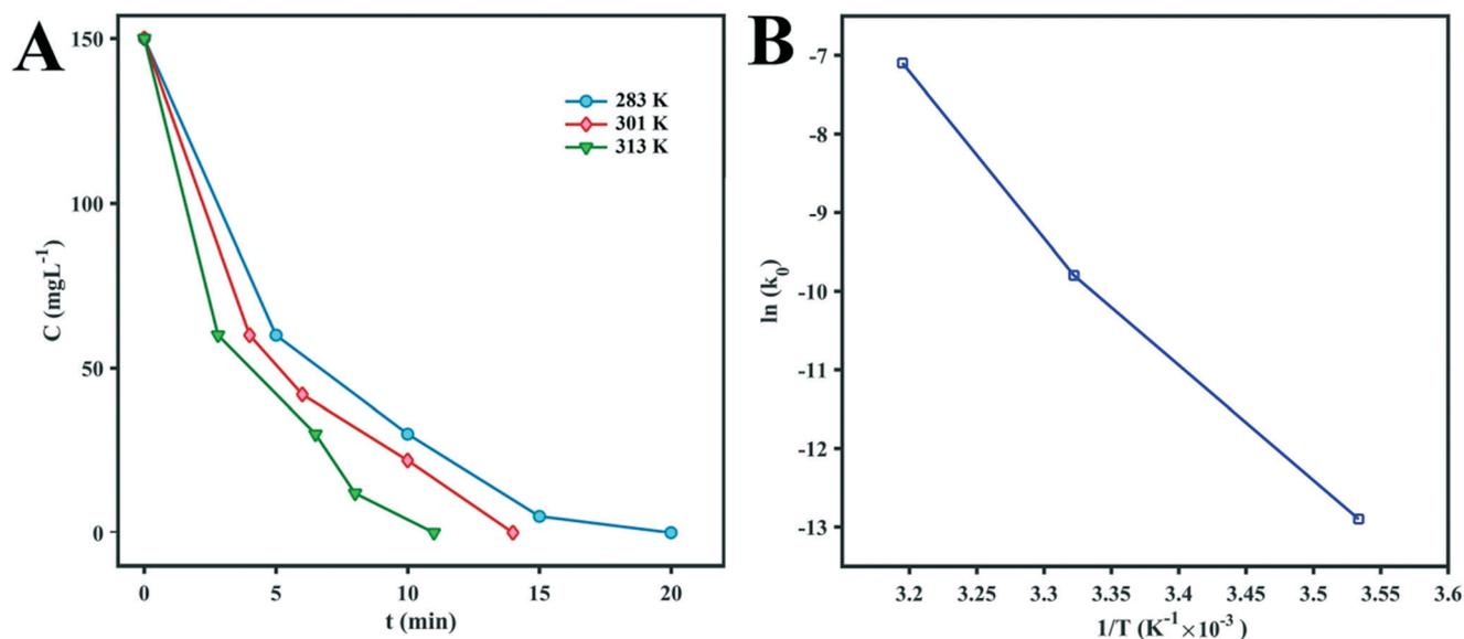
**Fig. 7** (A) Kinetic curves of MB degradation at different temperatures. (B) Arrhenius plot of  $\ln(k_0)$  vs.  $(1/T)$  for the photocatalytic degradation of MB by  $D_1$ .
