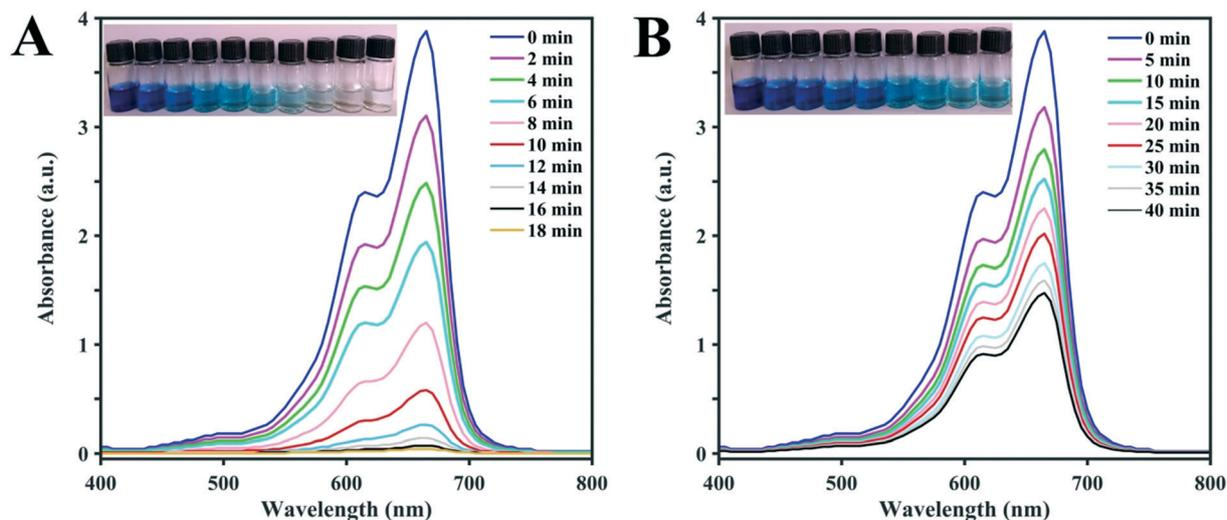
Fig. 5 The pictures and corresponding UV-vis spectra of MB solutions after photodegradation with visible light ( $\lambda > 420$  nm) for different times using (A)  $D_1$  and (B)  $D_2$  clusters as the photocatalysts.
