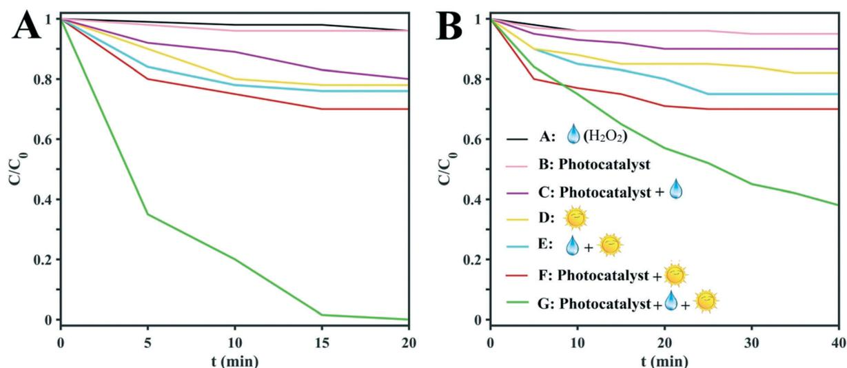
Fig. 4 Degradation over time of MB (as a model dye) under different conditions by D<sub>1</sub> (A) and D<sub>2</sub> (B). Black lines: H<sub>2</sub>O<sub>2</sub>/dark; pink lines: photocatalyst/dark; purple lines: H<sub>2</sub>O<sub>2</sub>/photocatalyst/dark; yellow lines: irradiation only; cyan lines: H<sub>2</sub>O<sub>2</sub>/irradiation; red lines: photocatalyst/irradiation; green lines: H<sub>2</sub>O<sub>2</sub>/photocatalyst/irradiation.
