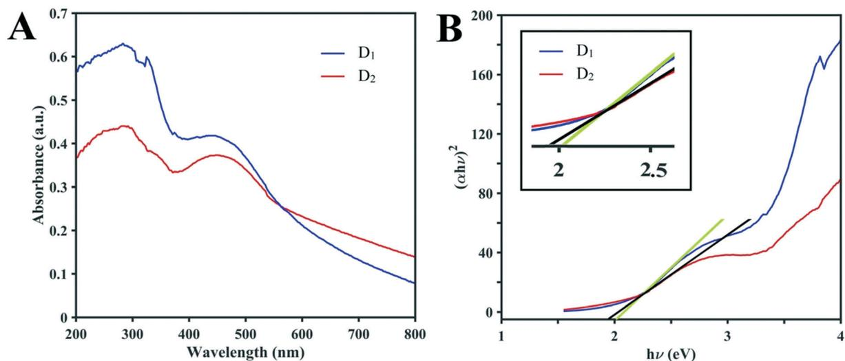
Fig. 6 (A) Solid-state UV-vis absorption spectra of  $D_1$  and  $D_2$  at ambient temperature. (B) Curves of the Kubelka–Munk function vs.  $E$  for  $D_1$  and  $D_2$  (the inset shows the magnification).
