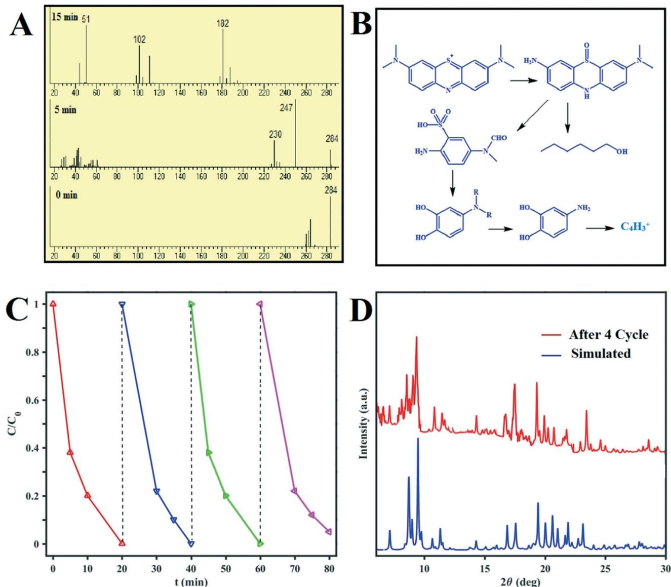
Fig. 8 (A) Mass spectra recorded of MB degradation at different reaction times. (B) Photocatalytic degradation pathway of MB.<sup>19</sup> (C) Recycling tests using  $D_1$  under sunlight irradiation for the photocatalytic degradation of MB. (D) Powder XRD patterns of  $D_1$  before and after four MB photocatalytic degradation cycles.
