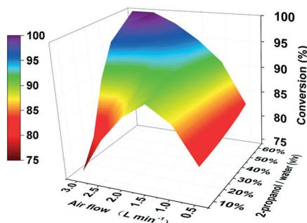
**Fig. 3** 3D bivariate coordinate system optimizing the TBCR. The air flow was studied in the range of 0.5 L min<sup>-1</sup> to 3.0 L min<sup>-1</sup>. The ratio of 2-propanol/water (v/v) was investigated from 10% to 60%.
