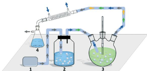
**Fig. 2** A schematic diagram of the TBCR system (not proportionally scaled). Area 1 is a pump unit. Area 2 is a buffer unit containing 2-propanol and water. Area 3 is a reaction unit, in which the temperature is set at 30 °C. Area 4 is a collection unit. Air, water, 2-propanol and acetone are shown as gray, blue, green and yellow arrows, respectively. Air paths are shown as light blue lines.
