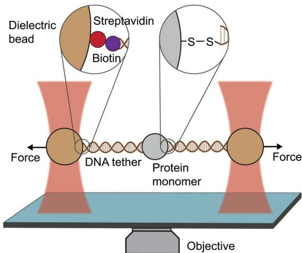
Fig. 4 Diagram representing a single-molecule experiment on a monomeric protein using optical tweezers (OT).
