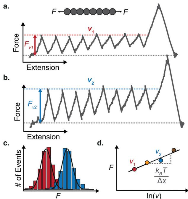
**Fig. 6** Force extension unfolding trajectories of a homopolyprotein pulled at (a) a low and (b) high pulling velocity. (c) The corresponding unfolding force histograms qualitatively show that the measured unfolding force increases with the pulling speed. (d) The average unfolding force at each pulling speed exhibits an approximate linear dependency with the natural logarithm of the pulling speed. The resulting gradient yields an estimate of the distance to the transition state ( $\Delta x$ ).
