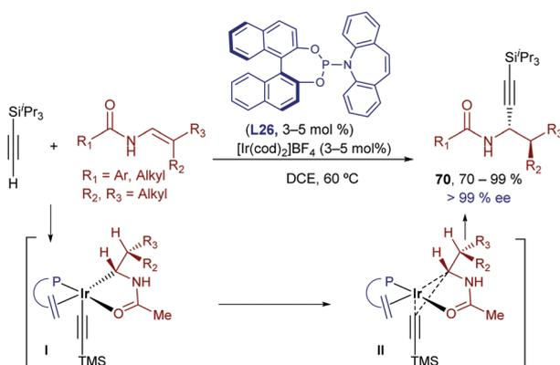
Scheme 45 An Ir-phosphoramidite catalyst for the hydroalkynylation of enamides.
