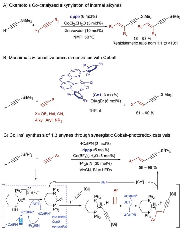
**Scheme 46** Cobalt-catalyzed hydroalkynylation reactions of alkynes [46C: SET stands for single electron transfer and 4CzIPN for 1,2,3,5-tetrakis(carbazol-9-yl)-4,6-dicyanobenzene; [Si] = <sup>i</sup>Pr<sub>3</sub>Si].
