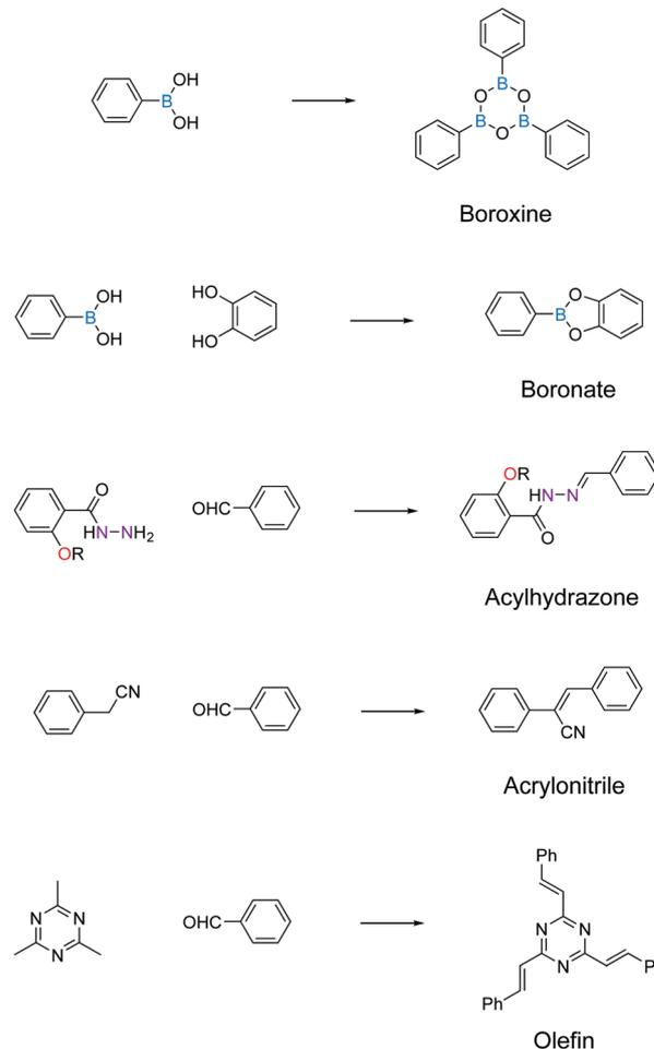
Fig. 2 Privileged covalent linkages for inducing solid-state light emission in 2D COFs.
