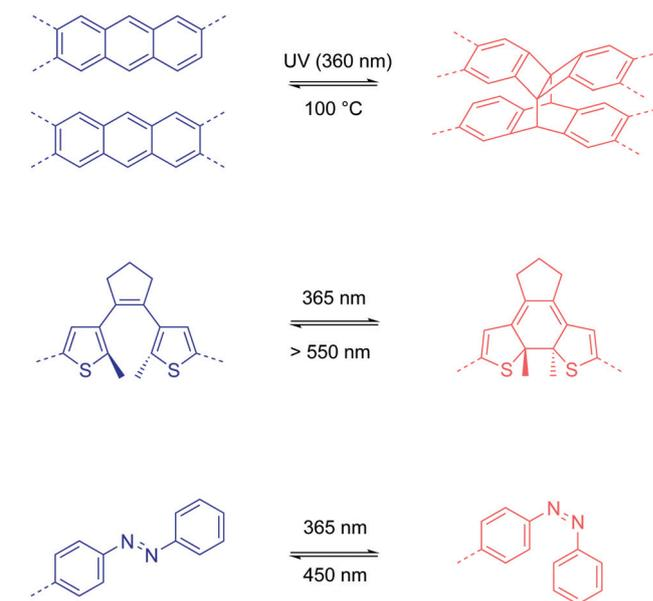
**Fig. 13** Photo-responsive functionalities in 2D COFs and their light-trigger isomerizations.
