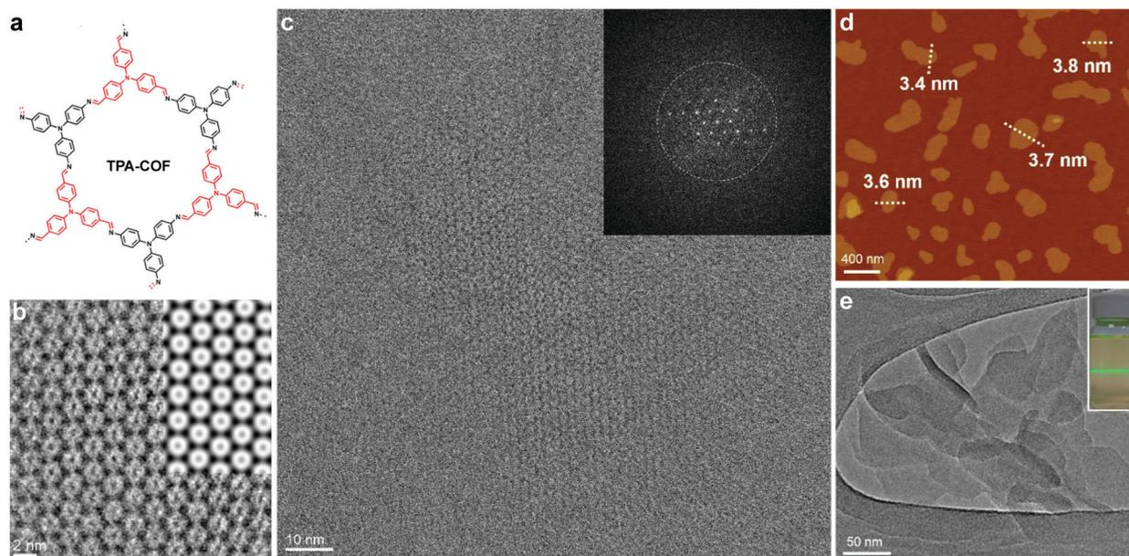
**Fig. 28** (a) TPA-COF reported by Zhang *et al.* (b) Enlarged high-resolution TEM of TPA-COFene denoised by using a Wiener filter. Inset: Simulated HRTEM image. (c) Low-dose high-resolution motion-corrected TEM image of TPA-COFene. Inset: Fast Fourier transform (FFT) of the TEM image. (d) AFM image of TPA-COFene. (e) TEM images of TPA-COFene. Inset: Photograph of the Tyndall effect of the TPA-COFene suspension. Reproduced with permission from ref. 19. Copyright 2017. American Chemical Society.
