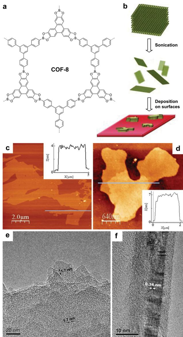
**Fig. 25** (a) Structure of COF-8. (b) Scheme of delamination of COF-8 and deposition on surfaces. AFM topographic images of COFene-8 on (c) mica and (d) silica substrates. TEM images showing the (e) in-plane and (f) out-of-plane crystallinity of COFene-8. Reproduced with permission from ref. 17. Copyright 2011. Wiley-VCH.
