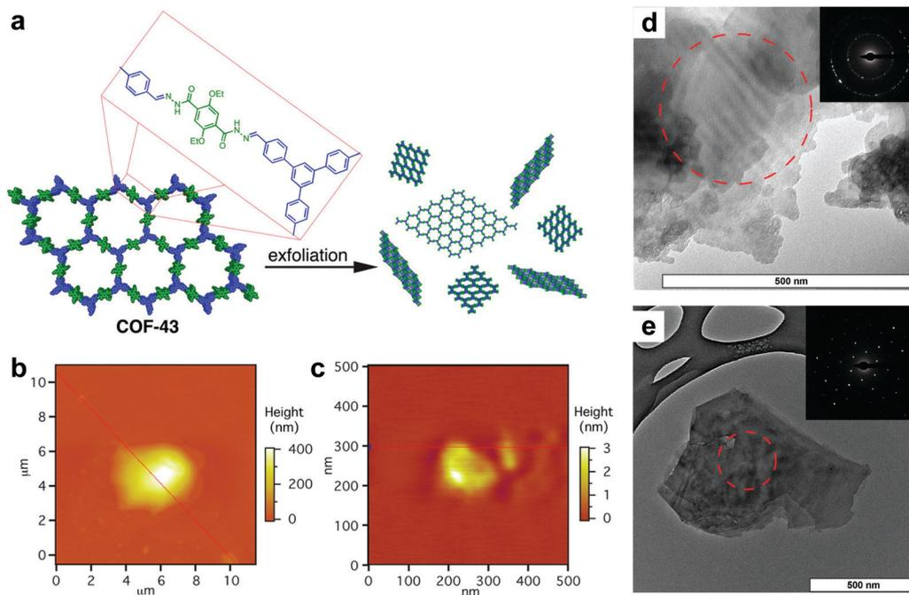
**Fig. 27** (a) Scheme of preparation of COFene-43. AFM images of COF-43 deposited onto freshly cleaved mica from (b) THF, which indicates particle sizes corresponding to hundreds of layers, and from (c) 1,4-dioxane, which shows platelets corresponding to few-layer structures. TEM images of a COF-43 suspension in (d) THF and (e) 1,4-dioxane (insets: SAED). Reproduced with permission from ref. 134. Copyright 2013. American Chemical Society.
