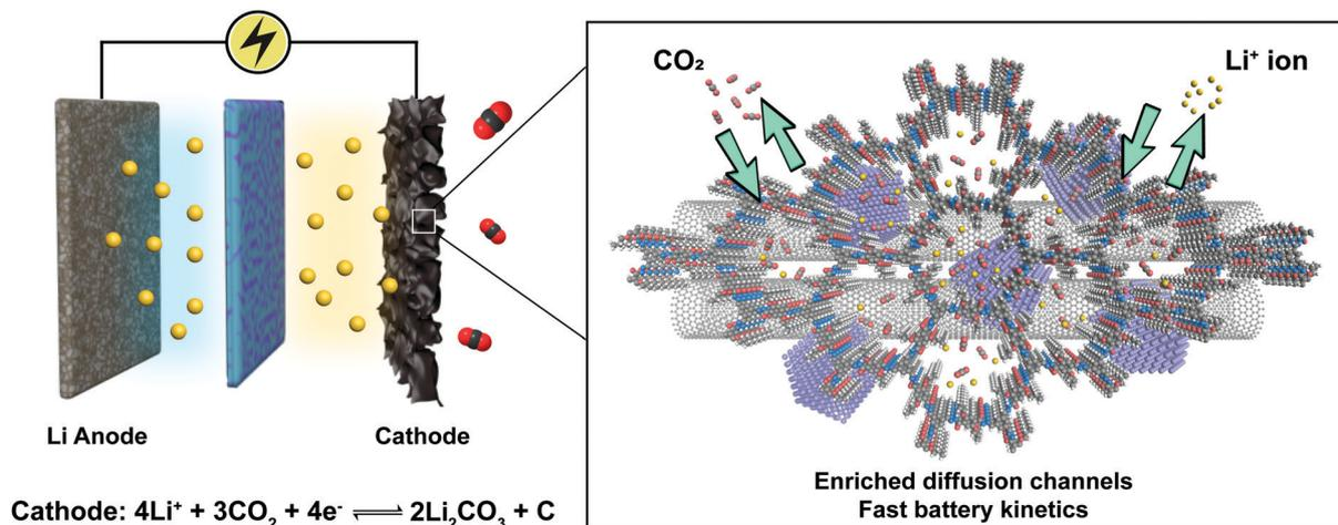
Fig. 22 Li-CO<sub>2</sub> battery based on the COF-incorporated cathode. Adapted with permission from ref. 93. Copyright 2019. Wiley-VCH.
