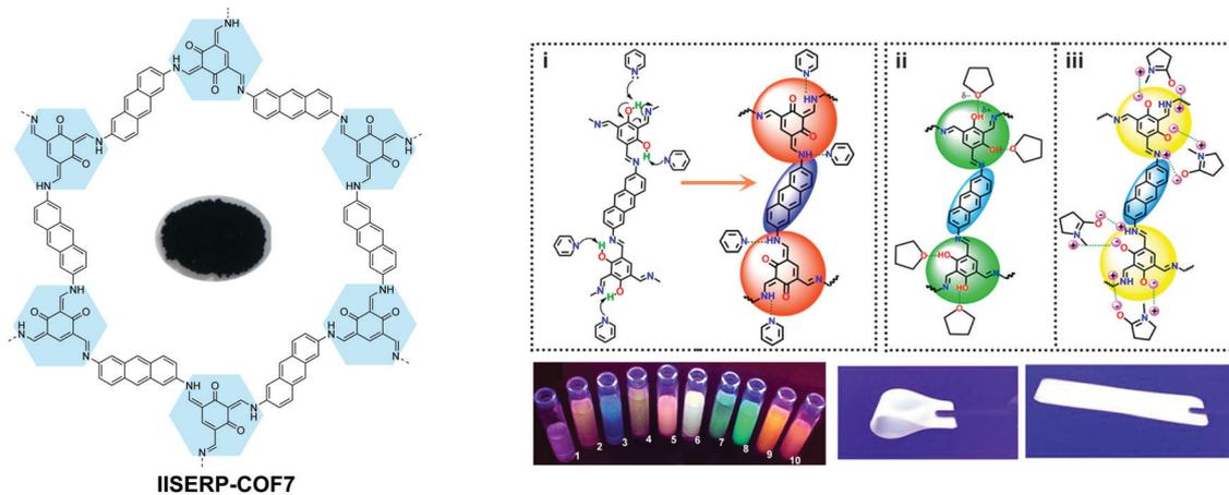
**Fig. 11** Solvatochromic emissive 2D COF based on enol–keto tautomerization. The proposed mechanism is shown for solvatochromic emission of the COF. COF dispersions in different solvents placed under a UV lamp. (1, THF; 2, 1,4-dioxane; 3, glyoxal; 4, pyridine; 5, DMA; 6, NMP; 7, ethanol; 8, formamide; 9, picoline; 10, DMF.) The COF in a flexible solid PMMA polymer matrix producing white emission. Reproduced with permission from ref. 63. Copyright 2017. American Chemical Society.
