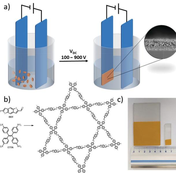
both depositions were carried out on FTO at 900 V for 2 min. Reproduced with permission from ref. 55. Copyright 2019, American Chemical Society.
