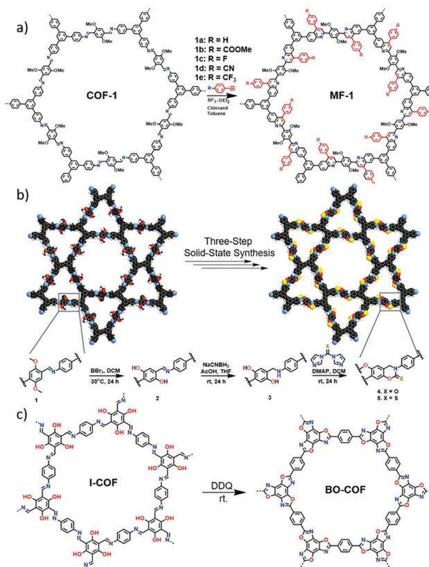
Fig. 7 (a) Post-synthetic modification of COFs *via* the aza-Diels–Alder reaction. Reproduced with permission from ref. 22. Copyright 2018, Springer Nature. (b) Synthesis of cyclic carbamate and thiocarbamate-linked COFs by a three-step solid-state synthesis process. Reproduced with permission from ref. 23. Copyright 2019, American Chemical Society. (c) The oxidative cyclization of I-COF into BO-COF. Reproduced with permission from ref. 24. Copyright 2019, American Chemical Society.
