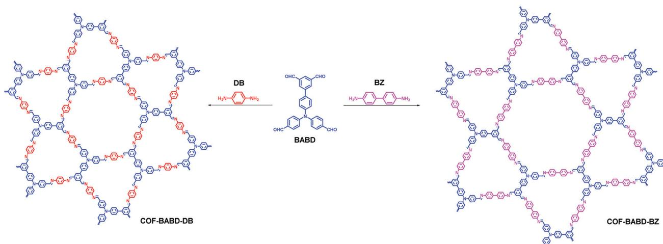
Fig. 22 Synthesis and structures of COF-BABD-DB and COF-BABD-BZ.<sup>125</sup>
