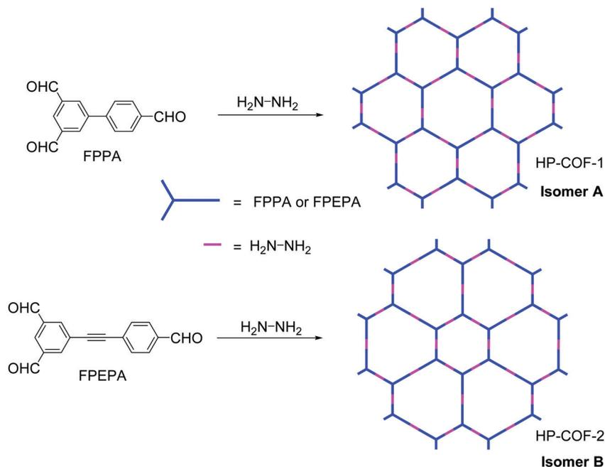
Fig. 21 Synthesis of HP-COFs.<sup>124</sup>
