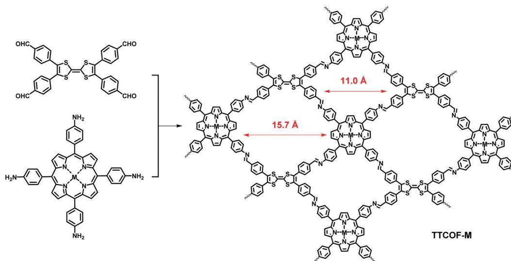
Fig. 18 Synthesis of **TTCOF-M**.<sup>120</sup>
