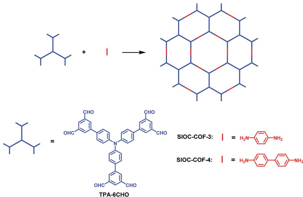
Fig. 29 Synthesis of COFs through the multiple-linking-site strategy.<sup>140</sup>
