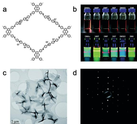
**Fig. 10** (a) Schematic of PyVg-COF. (b) Photos represent PyVg-COF dispersed in various solvents. Top, under sunlight; bottom, under 365 nm UV light. (c) Low magnification TEM image of PyVg-COF nanosheets. (d) SAED of the PyVg-COF nanosheet. Reproduced from ref. 155 with permission from the Royal Society of Chemistry, copyright 2019.
