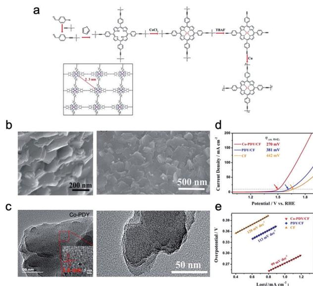
**Fig. 19** (a) Schematic illustration of the reaction of Co-PDY. (b) SEM images of Co-PDY/CF before (left) and after (right) the continuous electrocatalysis test for 10 h. (c) TEM images of Co-PDY/CF before (left) and after (right) the continuous electrocatalysis test for 10 h. (d) LSV curves of Co-PDY/CF, PDY/CF, and CF. (e) Tafel slope of Co-PDY/CF, PDY/CF, and CF. Reproduced from ref. 118 with permission from the Royal Society of Chemistry, copyright 2019.
