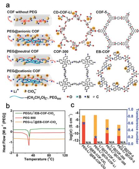
Fig. 13 (a) Schematic for Li<sup>+</sup> transport in neutral or ionic COFs, and chemical structures of CD-COF, COF-5, COF-300, and EB-COF. (b) DSC curves of PEG, PEG-Li<sup>+</sup>@EB-COF-ClO<sub>4</sub>, and PEG/Li<sup>+</sup>/EB-COF-ClO<sub>4</sub> (mechanical mixture sample). (c) The contribution of Li<sup>+</sup> conduction (red area) and anion conduction (orange area). Reproduced from ref. 205 with permission from American Chemical Society, copyright 2019.
