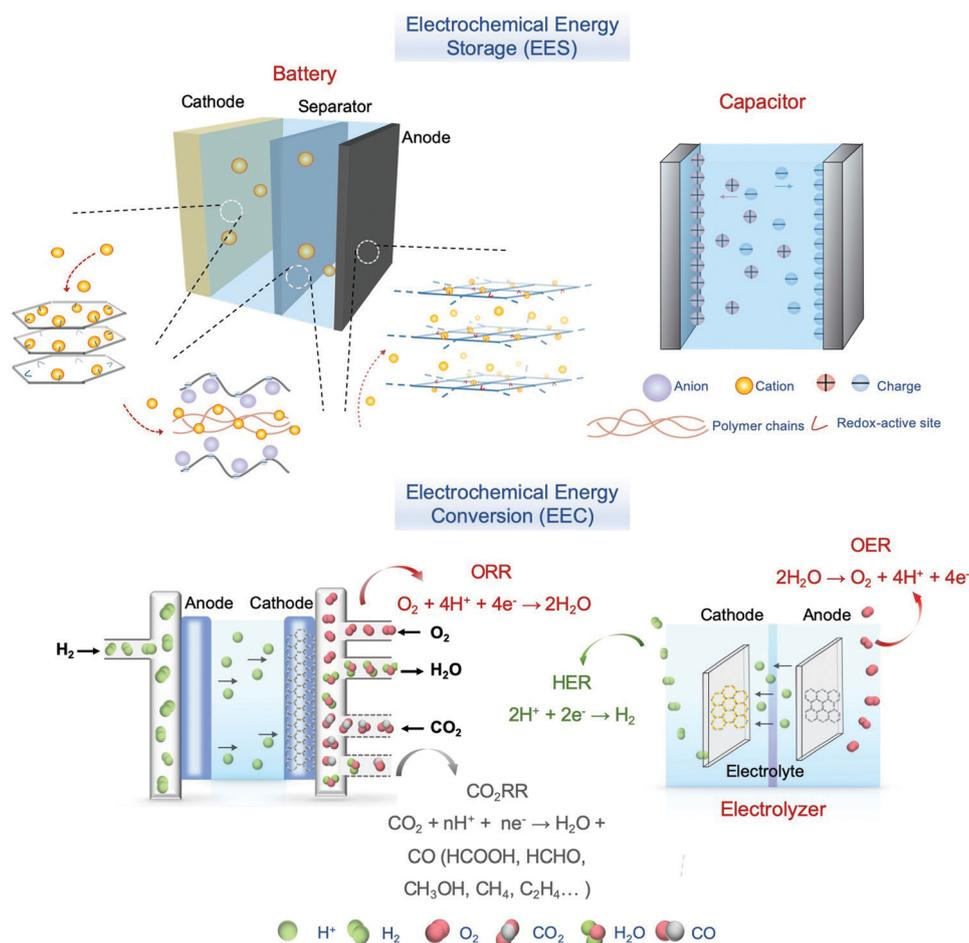
Fig. 3 Conceptual presentation of an integrated system of EES and EEC.
