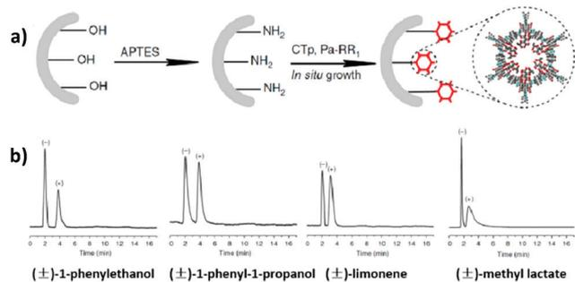
Fig. 23 (a) The *in situ* growth approach by injecting a solution of CTP and Pa-1 into the amino-modified capillary column. (b) Gas chromatograms of (±)-1-phenylethanol, (±)-1-phenyl-1-propanol, (±)-limonene and (±)-methyl lactate on a CTPa-1-bound capillary column. Adapted from ref. 28 with permission from Nature Research, copyright 2016.
