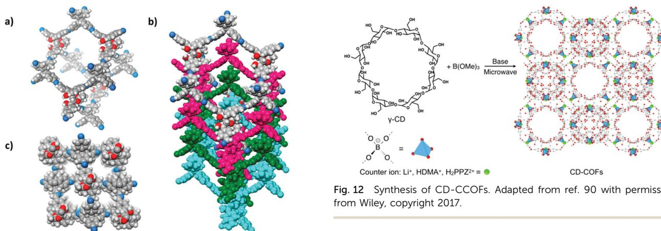
Fig. 12 Synthesis of CD-COFs. Adapted from ref. 90 with permission from Wiley, copyright 2017.
