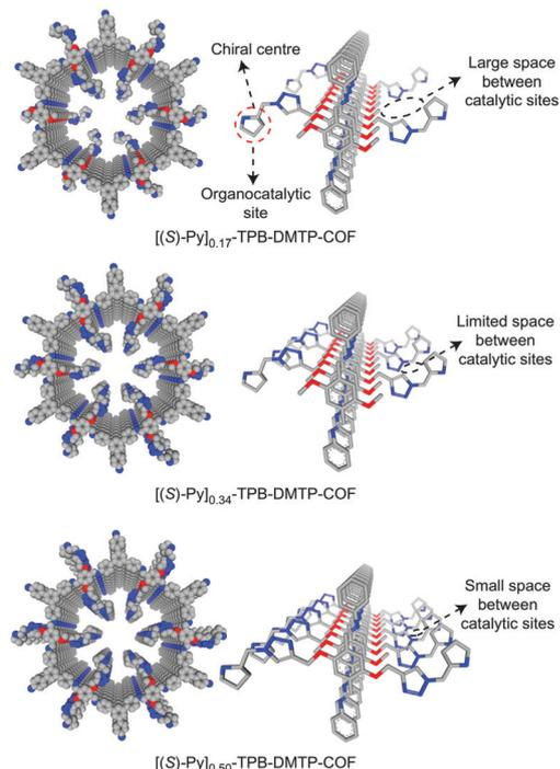
Fig. 16 Channel-wall structure of [(S)-Py]<sub>x</sub>-TPB-DMTP-COFs ( $x = 0.17, 0.34$  and  $0.50$ ). Adapted from ref. 73 with permission from Nature Research, copyright 2017.
