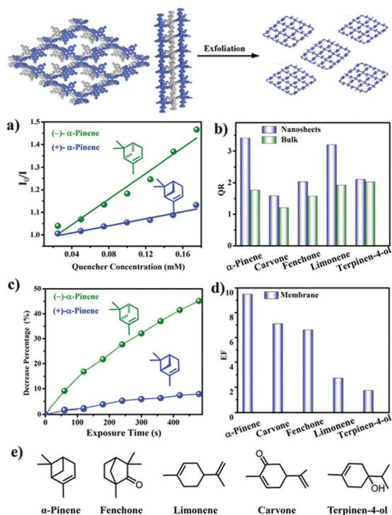
Fig. 27 The illustration of CCOF 7 exfoliation and the applications in fluorescence recognition. (a) Stern–Volmer plots of 7-NS upon titration of  $\alpha$ -pinene in MeCN. (b) Enantioselective quenching ratio for several terpenes. (c) Decrease percentage upon exposure to  $\alpha$ -pinene for 7@PVDF. (d) Enantioselective fluorescence decrease ratio for several vapors. (e) Chemical structures of terpenes. Reproduced from ref. 87 with permission from the American Chemical Society, copyright 2019.
