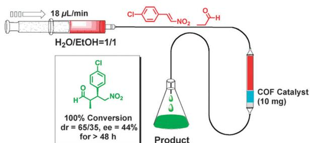
Fig. 14 The flow reaction system based on the [Pyr]<sub>25</sub>-H<sub>2</sub>P-COF column for Michael addition reaction. Adapted from ref. 72 with permission from the Royal Society of Chemistry, copyright 2014.
