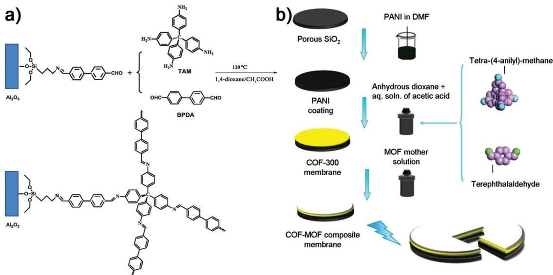
Fig. 6 (a) Fabrication of the COF-320 membrane on modified porous  $\text{Al}_2\text{O}_3$  (reproduced from ref. 69 with permission from Royal Society of Chemistry, Copyright 2015). (b) Fabrication of the COF-300 membrane and further COF–MOF composite membranes on modified porous  $\text{SiO}_2$  (reproduced from ref. 70 with permission from American Chemical Society, Copyright 2016).
