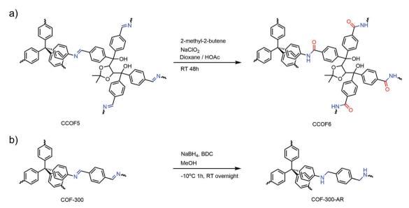
Fig. 11 Linkage transformation (a) from imine to amide in CCOFs and (b) from imine to amine in COF-300-AR.
