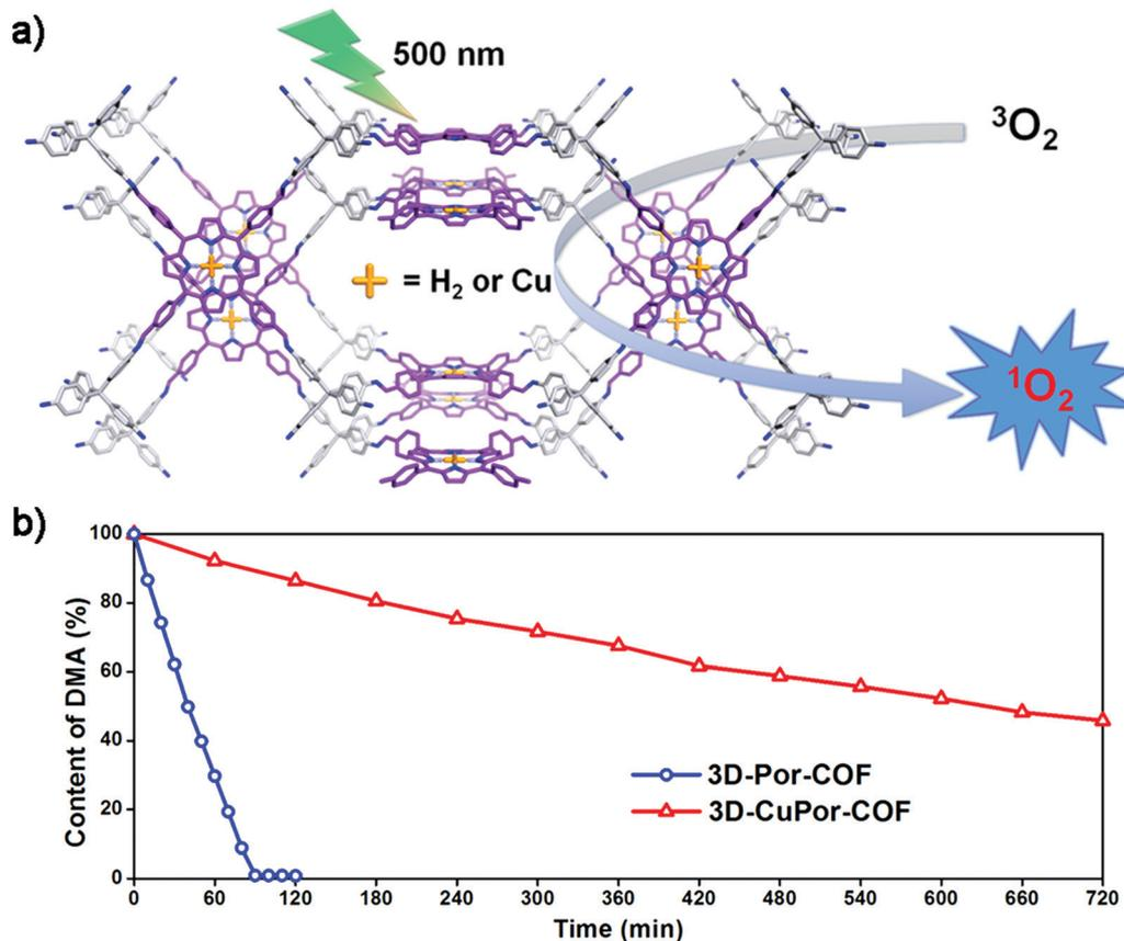
Fig. 18 (a) Schematic representation of 3D-Por-COF and 3D-CuPor-COF as heterogeneous catalysts for generating singlet oxygen. (b) Concentration irradiation time plots of 9,10-dimethylantracene (DMA) (reproduced from ref. 75 with permission from American Chemical Society, Copyright 2017).
