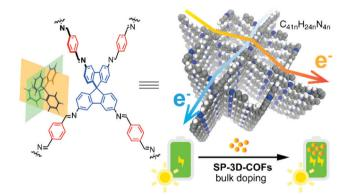
**Fig. 21** Schematic representation of SP-3D-COF as PSC doping materials (reproduced from ref. 49 with permission from American Chemical Society, Copyright 2018).
