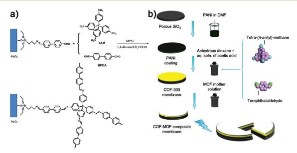
Fig. 6 (a) Fabrication of the COF-320 membrane on modified porous Al<sub>2</sub>O<sub>3</sub> (reproduced from ref. 69 with permission from Royal Society of Chemistry, Copyright 2015). (b) Fabrication of the COF-300 membrane and further COF-MOF composite membranes on modified porous SiO2 (reproduced from ref. 70 with permission from American Chemical Society, Copyright 2016).
