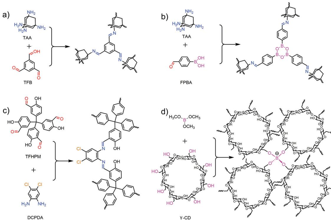
**Fig. 8** (a) Base sites generated in BF-COFs. (b) Acid and base sites generated in DL-COFs. (c) Salphen groups generated in JUC-508 and JUC-509. (d) Anionic tetrakis(spiroborate) moieties generated in CD-COFs.
