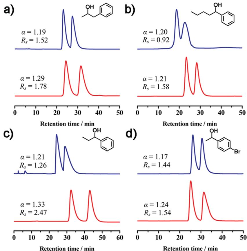
Fig. 16 Separation performance of racemic alcohols with CCOF 5 (blue line) and 6 (red line) as the stationary phase of chromatography (reproduced from ref. 50 with permission from American Chemical Society, Copyright 2018).
