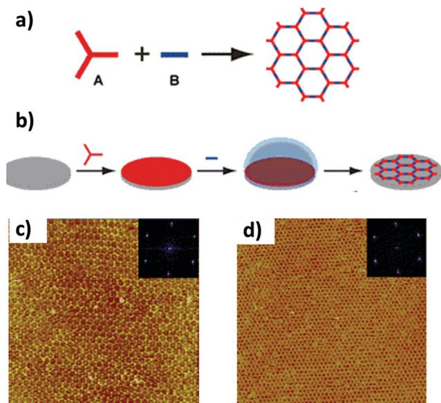
**Fig. 8** (a) Scheme of the condensation reaction of two precursors A and B to yield the formation of a COF. (b) Scheme diagram for a solid–vapour interface reaction. Large-scale STM images ( $100 \times 100 \text{ nm}^2$ ) of (c) SCOF-IC1 and (d) SCOF-LZU1. The insets depict the corresponding FFT spectra of the STM images. Reproduced from ref. 33 with permission from the American Chemical Society, copyright 2013.
