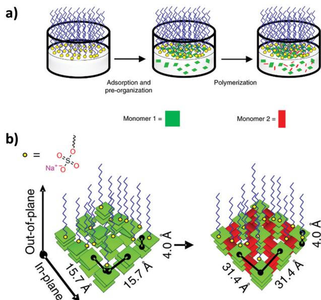
**Fig. 9** (a) Schematic of the synthetic procedure on the air/water interface assisted by a surfactant layer. (b) Schematic of the preorganization of the first building block followed by CON formation upon addition of the second building block. Reproduced from ref. 37 with permission from Springer Nature, copyright 2019.
