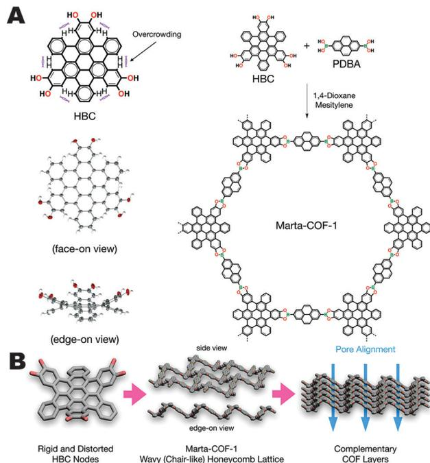
**Fig. 15** (A) Synthesis and structure of Marta-COF-1, and the contorted hexabenzocoronene monomer units. (B) The wavy 2D sheets of Marta-COF-1 are self-complementary resulting in excellent crystallinity and pore alignment. Reproduced from ref. 13 with permission from ACS Publications, copyright 2019.
