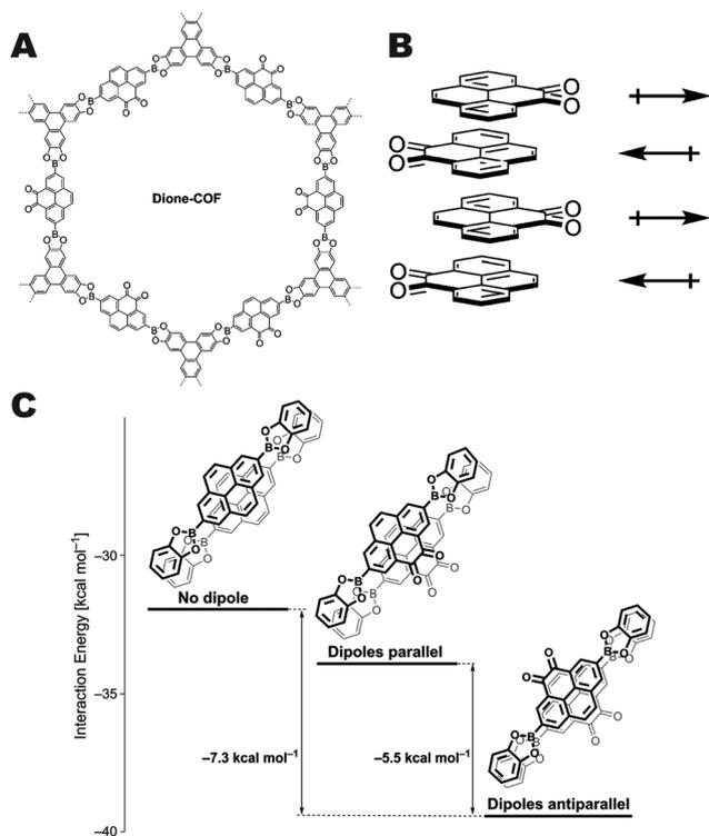
**Fig. 11** (A) Structure of dione-COF, (B) schematic of the dipole canceling arrangement of the monomers, and (C) relative interaction energies of the dione-COF linkers in both the parallel and antiparallel arrangement in comparison with the native pyrene monomer. Reproduced from ref. 12 with permission from the Royal Society of Chemistry, copyright 2016.
