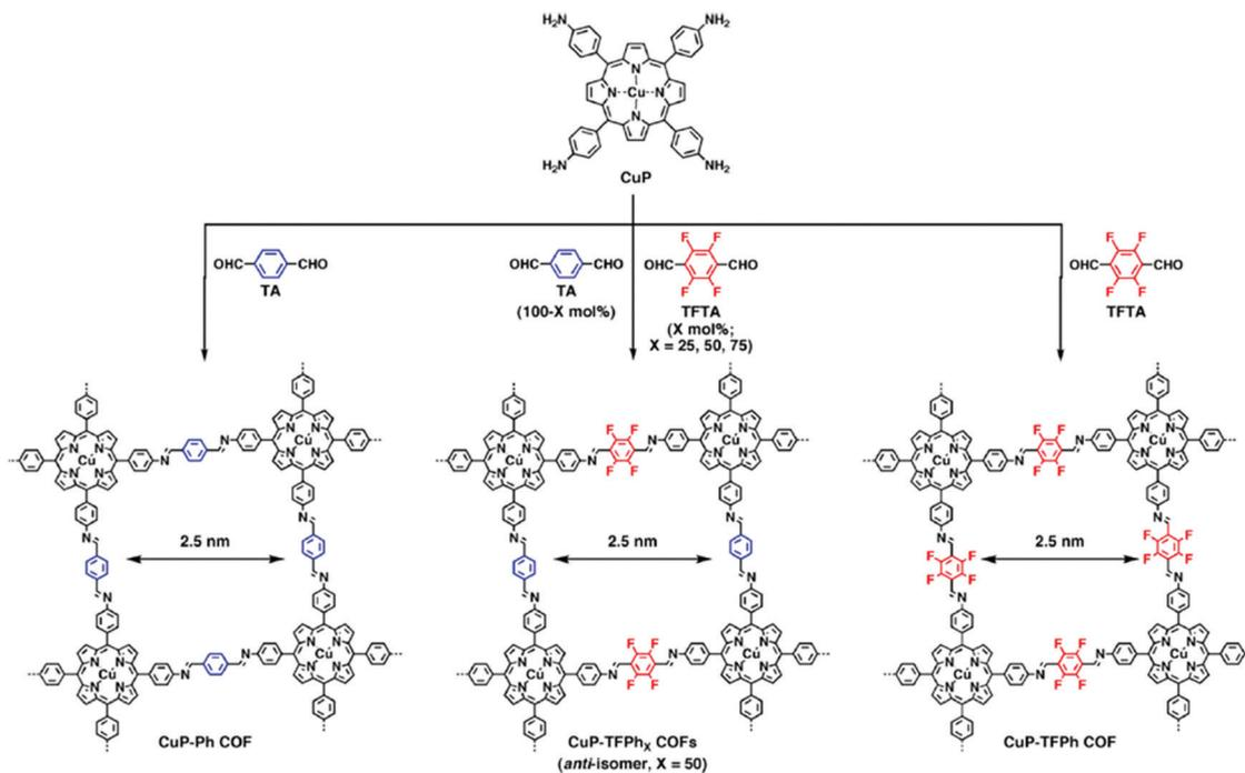
Fig. 4 COFs synthesized containing aromatic linkers of different electron densities. Variation of the monomer feed ratio can strongly affect the COF crystallinity and surface area. In this case, a 1:1 ratio of TA and TFTA results in the most crystalline structure because of the interlayer interactions between electron rich and poor rings. Reproduced from ref. 7 with permission from ACS Publications, copyright 2013.
