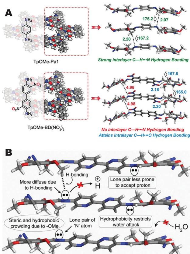
Fig. 16 (A) Representation of TpOME-Pa1 and TpOME-BD(NO<sub>2</sub>)<sub>2</sub> with hydrogen bonding between neighbouring COF layers and (B) the structural origin of the interlayer hydrogen bonding in TpOME-BPy. Reproduced from ref. 44 Wiley-VCH Verlag GmbH & Co., copyright 2018.
