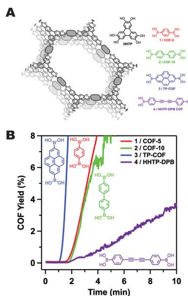
Fig. 3 (A) A series of boronate ester COFs with varying  $\pi$ -surface sizes. (B) Rates of COF formation observed through turbidity measurements. Figure adapted from ref. 35 with permission from the Royal Society of Chemistry, copyright 2015.
