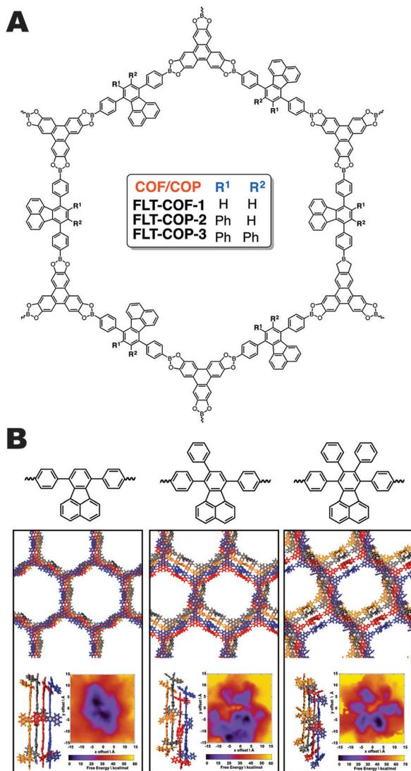
**Fig. 14** (A) Structure of FLT-COFs and covalent organic polymers (COPs). (B) Molecular dynamics (MD) simulations of the FLT-COF structures illustrating that the added steric hindrance from additional phenyl rings could disrupt the eclipsed packing of the COF layers. This disruption is attributed to the tri- and tetraphenylfluoranthene monomers inability to form crystalline COF structures. Reproduced from ref. 14 with permission from ACS Publications, copyright 2017.
