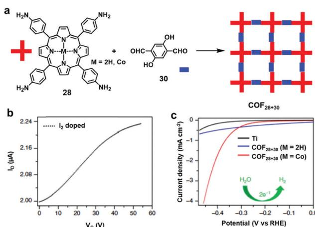
Fig. 23 (a) Synthesis of  $\text{COF}_{28+30}$  from monomers **28** and **30**; (b) transfer curve of a thin film transistor employing  $\text{COF}_{28+30}$  ( $M = 2H$ ) as an active semiconducting layer at a source to drain voltage of  $-40 \text{ V}$  after doping with iodine; (c) hydrogen evolution reaction polarization plots of blank titanium foil (black) and multilayer  $\text{COF}_{28+30}$  ( $M = \text{Co}^{\text{II}}$ ). Reproduced from ref. 43.
