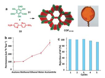
Fig. 25 (a) Synthesis of  $COF_{31+33}$  at the liquid-liquid interface and its modelling and optical image; (b) permeances of pure solvents for  $COF_{31+33}$ thin film; (c) recyclability of the COF<sub>31+33</sub> thin film for acid fuchsin (AF) rejection over 24 h for 5 cycles. Reproduced from ref. 51 with permission, Copyright 2017, The American Chemical Society.
