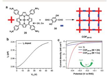
Fig. 23 (a) Synthesis of COF<sub>28+30</sub> from monomers **28** and **30**; (b) transfer curve of a thin film transistor employing  $COF_{28+30}$  (M = 2H) as an active semiconducting layer at a source to drain voltage of -40 V after doping with iodine; (c) hydrogen evolution reaction polarization plots of blank titanium foil (black) and multilayer COF<sub>28+30</sub> (M = Co<sup>II</sup>). Reproduced from
