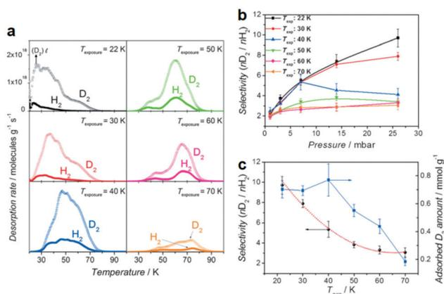
Fig. 18 (a)  $\text{H}_2$  and  $\text{D}_2$  TDS of 26 mbar (1:1  $\text{H}_2/\text{D}_2$  mixture) loading on Py@COF-1 with a heating rate of  $0.1 \text{ K s}^{-1}$ . (b) Equimolar mixture selectivity as a function of loading pressure for different temperatures. (c)  $T_{\text{exp}}$  dependence of the maximum selectivity and corresponding adsorbed  $\text{D}_2$  amount. Reproduced with permission from ref. 89. Copyright 2013, Wiley-VCH.
