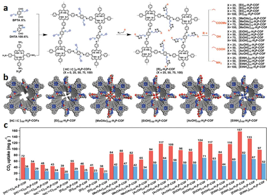
Fig. 14 (a) Schematic of pore surface engineering of imine-linked COFs with various functional groups *via* click reactions; (b) pore structures of COFs with different functional groups; (c) CO<sub>2</sub> adsorption capacity of the COFs at 273 (red) and 298 K (blue) and 1 bar. Reproduced with permission from ref. 155. Copyright 2015, American Chemical Society.
