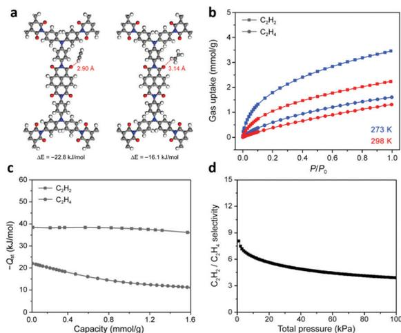
**Fig. 16** (a) Optimized binding sites and binding energies for acetylene and ethylene within PAF-110. (b) Acetylene and ethylene adsorption isotherms for PAF-110 at 273 K (blue symbols) and 298 K (red symbols). (c)  $Q_{st}$  curves for acetylene and ethylene. (d) Acetylene/ethylene adsorption selectivity of PAF-110 at 298 K, as determined from ideal adsorbed solution theory. Reproduced with permission from ref. 96. Copyright 2018, American Chemical Society.
