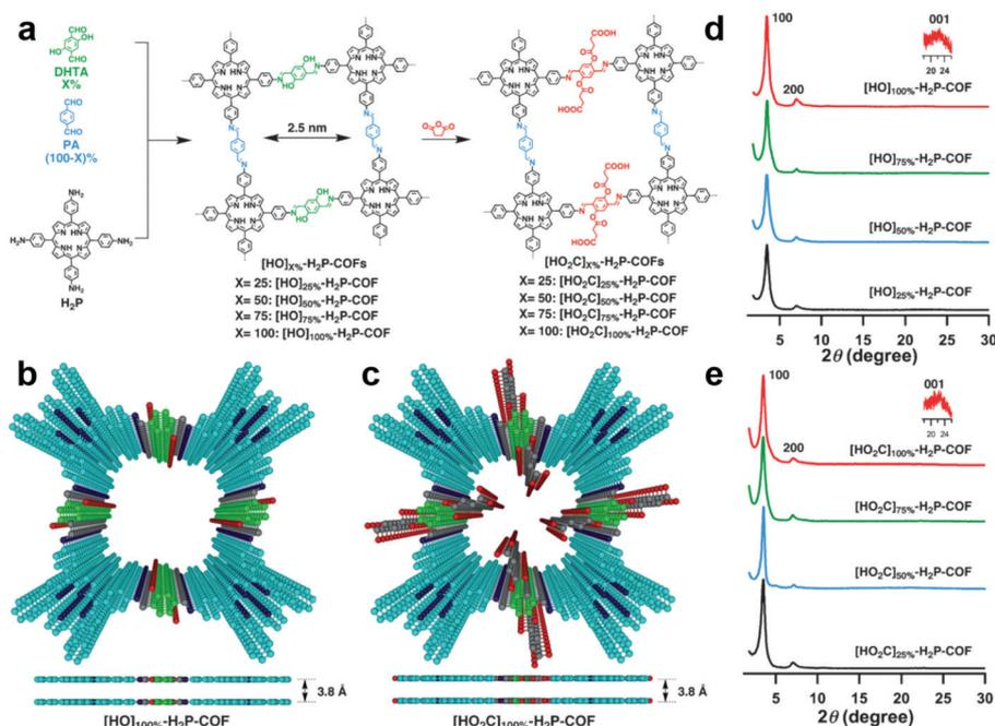
Fig. 7 (a) Synthesis of  $[\text{HO}_2\text{C}]_x\text{-H}_2\text{P-COFs}$  with channel walls functionalized with carboxylic acid groups through the ring opening reaction. Top views of (b)  $[\text{HO}]_{100\%}\text{-H}_2\text{P-COF}$  and (c)  $[\text{HO}_2\text{C}]_{100\%}\text{-H}_2\text{P-COF}$ . XRD patterns of (d)  $[\text{OH}]_x\text{-H}_2\text{P-COFs}$  and (e)  $[\text{HO}_2\text{C}]_x\text{-H}_2\text{P-COFs}$ . Reproduced with permission from ref. 106. Copyright 2017, Wiley-VCH.
