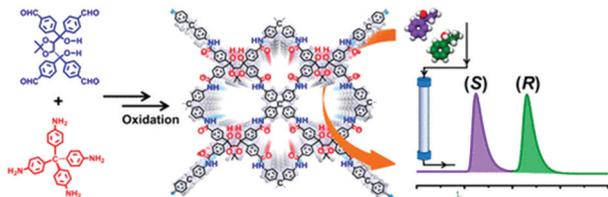
Fig. 30 Schematic illustrations for the synthesis of 3D chiral COFs and their use as CSPs for HPLC. Reproduced with permission from ref. 258. Copyright 2019, American Chemical Society.
