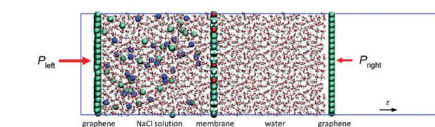
Fig. 22 The simulation system for water desalination through COF membranes (C: cyan; O: red; H: white; Na<sup>+</sup>: blue; Cl<sup>-</sup>: cyan). Reproduced with permission from ref. 221. Copyright 2017, Royal Society of Chemistry.
