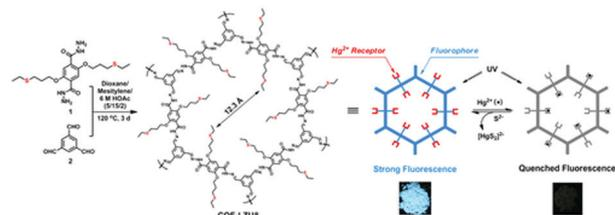
Fig. 24 Schematic illustration of the synthesis route of COF-LZU8 and its application for  $\text{Hg}^{2+}$  detection and removal. Reproduced with permission from ref. 224. Copyright 2016, American Chemical Society.
