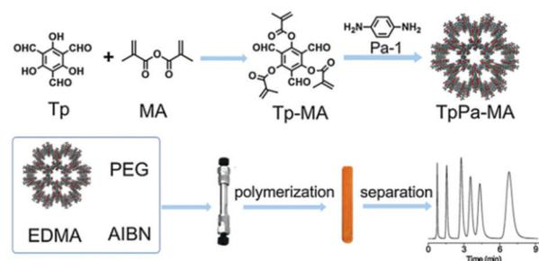
Fig. 28 Schematic illustration of the fabrication of the poly(TaPa-MA-*co*-EDMA) monolith for HPLC. Reproduced with permission from ref. 95. Copyright 2017, Elsevier.
