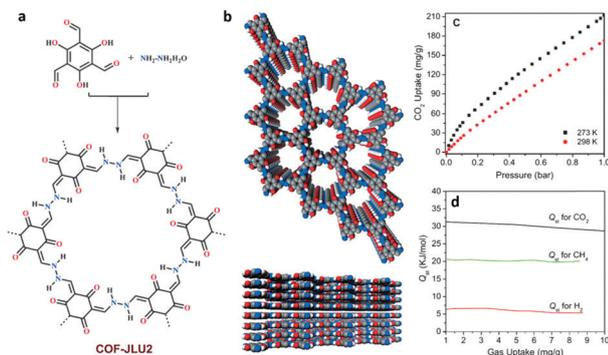
Fig. 13 (a) Schematic representation of the synthesis of COF-JLU2. (b) Top and side views of the AA stacking structure of COF-JLU2. (c)  $\text{CO}_2$  sorption measurements for COF-JLU2. (d) Isothermic heats of adsorption for COF-JLU2. Reproduced with permission from ref. 150. Copyright 2015, Wiley-VCH.
