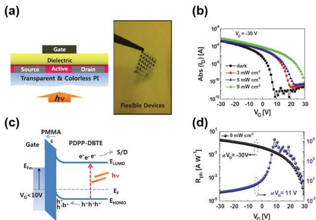
Fig. 23 (a) Schematic illustration of PDPP-DBTE-based OPTs and photograph of devices fabricated on flexible substrates; (b)  $I_D \times V_{GS}$  characteristics in the dark and under illumination at various light intensities; (c) energy band diagram of PDPP-DBTE-based OPTs under illumination conditions with a negative  $V_{GS}$ ; and (d) photoresponsivity and sensitivity as a function of  $V_{GS}$  (reprinted with permission from Kim *et al.*,<sup>187</sup> copyright 2014, Elsevier).
