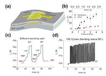
Fig. 30 (a) Schematic representation of a P3HT based OFET flexible device. (b) Comparison of P3HT and pentacene device current response for different pressure and strain conditions applied. (c) Distinct current response for a wide range of device bending conditions from 180 to 90 degree. (d) Repeatable (100 times) current response of the device under 90 degree bending radius strain condition (reprinted with permission from Loi et al., 246 copyright 2013, IEEE).
