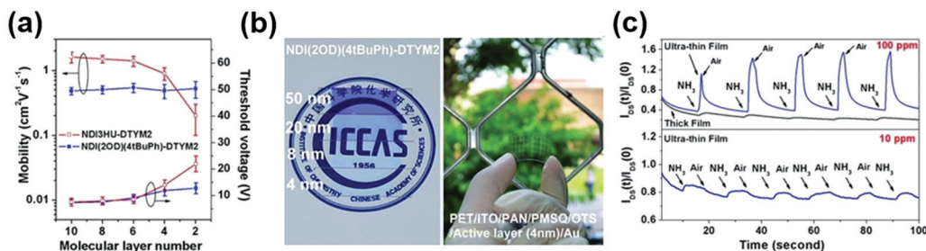
Fig. 15 (a) Relationship between transistor parameters and the thickness of the active layers; (b) demonstrating the transparent properties of the as-fabricated device; (c) ammonia-sensing properties of thick and ultrathin film-based devices (reprinted with permission from Zhang et al. , 118 copyright 2013, Wiley-VCH).
