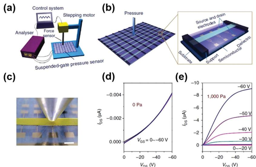
Fig. 8 (a) Schematic illustration of the experimental set-up of suspended-gate OFET pressure sensors; (b) an OFET array and magnified view of the device geometry; (c) optical image of a suspended-gate OFET (scale bar corresponds to 1 mm);  $I_D$ - $V_{DS}$  curves of the transistors recorded at (d) 0 Pa and (e) 1000 Pa (reprinted with permission from Zang *et al.*,<sup>85</sup> copyright 2015, Nature).
