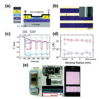
Fig. 20 (a) Schematic illustration of a PQT-12/C[8]A NF-based OFET device; (b) optical image along with SEM (inset) image of nanofibers; (c) transient response toward n-hexane, ethanol, and toluene vapors; (d) effect of bending radius on both "off" and "on" current of the device; (e) real-time demonstration of the OFET sensor for an IoT-based monitoring system (reprinted with permission from Kweon  $et\ al.$ , <sup>123</sup> copyright 2019, Royal Society of Chemistry).
