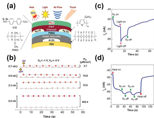
Fig. 33 (a) Schematic representation and (b) photo-response of the bottom contact OFET device with a dual polymer gate dielectric. Multi-sensing device response toward (c)  $N_2$  and light, (d) heat and  $N_2$  stimulants (reprinted with permission from Song *et al.*,<sup>240</sup> copyright 2017, Nature).
