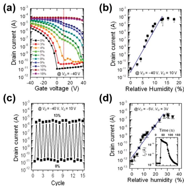
Fig. 21 (a) Effect of different humidity levels on the transfer behavior of an OFET device. At  $V_D = -40$  V and  $V_G = 10$  V, (b) relationship between the device drain current and humidity, and (c) repeatable behavior of the device toward 13% humidity. (d) Flexible OFET device behavior and (inset) transient response toward different humidity levels at  $V_D = -5$  V and  $V_G = 3$  V (reprinted with permission from Park *et al.*,<sup>171</sup> copyright 2013, American Chemical Society).
