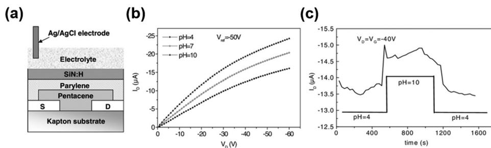
Fig. 25 (a) Schematic representation of flexible OFET device, (b) output characteristics and (c) transient response of device toward pH = 4, 7, and 10 (reprinted with permission from Diallo *et al.*,<sup>214</sup> copyright 2008, American Institute of Physics).
