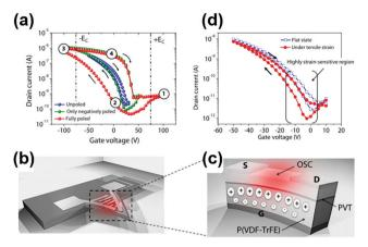
(a) Comparison of transfer characteristics and associated hysteresis behavior for different poling conditions. (b) Effect of strain and (c) corresponding impact on the dipole properties of the P(VDF-TrFE) layer. (d) Change in device transfer characteristics under applied tensile strain conditions (reprinted with permission from Thuau et al., <sup>174</sup> copyright 2016, Nature).
