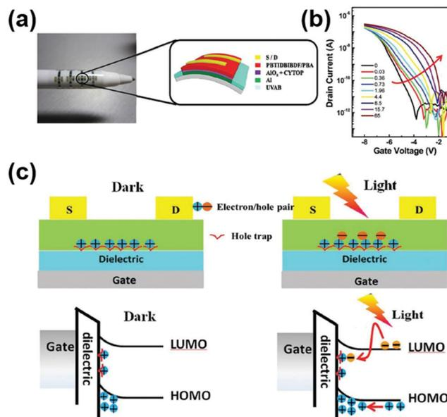
Fig. 24 (a) Flexible PBTIDBIBDF-based OPTs fabricated in the BGTC architecture; (b)  $I_D \times V_{GS}$  characteristics of OPTs under various illumination intensities ( $V_{DS} = -5 \text{ V}$ ); and (c) schematic illustration of the OPTs and energy band diagrams elucidating the photoresponse behavior (reprinted with permission from Wang *et al.*,<sup>201</sup> copyright 2019, Wiley-VCH).
