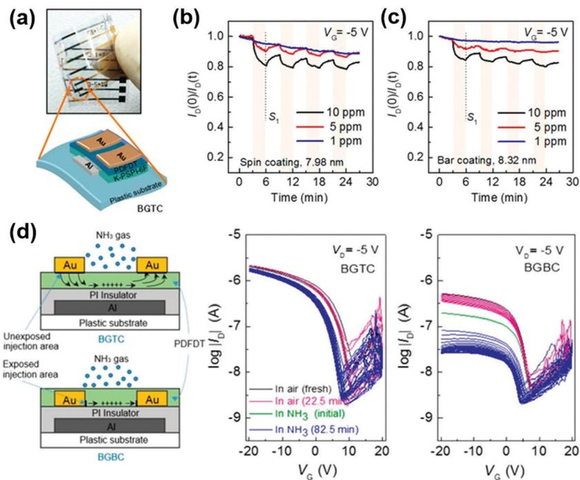
**Fig. 18** (a) Schematic representation of PDFDT OFET sensor arrays on flexible substrates; (b) spin-coated and (c) bar-coated OFET sensing behavior to 10, 5, and 1 ppm ammonia gas; (d) ammonia-sensing mechanism and associated transfer behavior in BGTC and BGBC device geometry (reprinted with permission from Yawson *et al.*,<sup>121</sup> copyright 2017, American Chemical Society).
