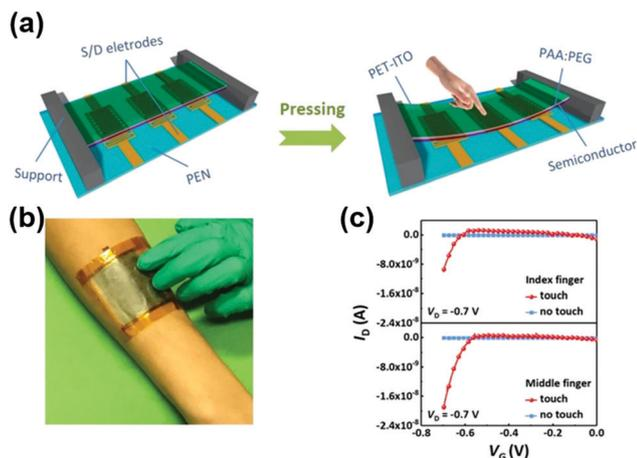
Fig. 10 (a) Schematics of the suspended-gate OFET pressure sensors, before and after the pressing of the flexible (suspended) gate structure; (b) photograph of the OFET sensor array affixed to a human arm; and (c) pressure-sensing response of the devices when touched using the index and middle fingers (reprinted with permission from Liu *et al.*,<sup>87</sup> copyright 2019, Wiley-VCH).
