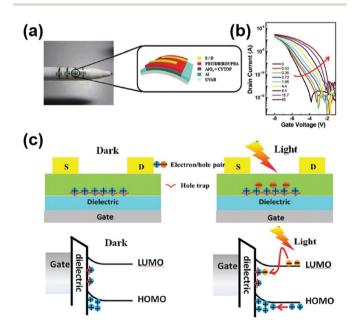
Fig. 24 (a) Flexible PBTIDBIBDF-based OPTs fabricated in the BGTC architecture; (b)  $I_{\rm D} \times V_{\rm GS}$  characteristics of OPTs under various illumination intensities ( $V_{DS} = -5$  V); and (c) schematic illustration of the OPTs and energy band diagrams elucidating the photoresponse behavior (reprinted with permission from Wang et al., 201 copyright 2019, Wiley-VCH).
