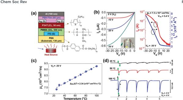
Fig. 12 (a) Schematic representation, (b) output and transfer characteristics of the fabricated OFET thermal sensor, (c) relation between charge carrier mobility of the sensor and ambient temperature, (d) drain current response of the sensor for different temperatures (reprinted with permission from Song et al., 98 copyright 2017, American Chemical Society).
