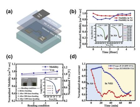
Fig. 17 (a) Schematic representation of a P-29-DPP-SVS-based OFET device. Relationship between the normalized mobility and the effect of (b) air and  $N_2$  ambient, and (c) bending radius of the flexible OFET device. (d) Ammonia-sensing behavior of both p-type P-29-DPP-SVS and n-type (P(NDI2OD-T2)) materials (reprinted with permission from Ryu *et al.*, <sup>120</sup> copyright 2015, Elsevier B.V.).
