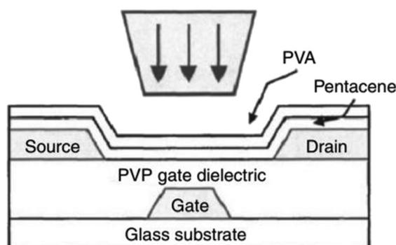
**Fig. 6** Schematic illustration showing OFETs fabricated on a glass substrate and operating as free-standing pressure sensors (reprinted with permission from Darlinski *et al.*,<sup>81</sup> copyright 2005, American Institute of Physics).
