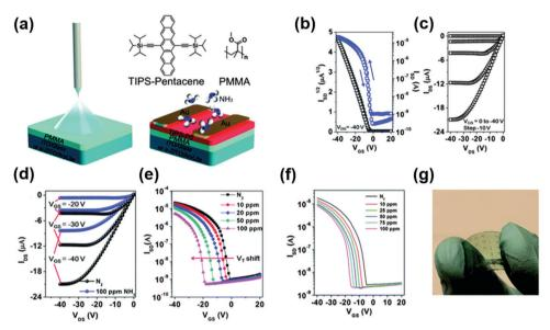
Fig. 16 (a) Schematic representation; (b and c) electrical characteristics; (d and e) ammonia-sensing behavior of the as-fabricated TIPS-pentacene on a glass substrate; and (f and g) ammonia-sensing behavior of the same device on a flexible substrate (reprinted with permission from Yu et al., 119 copyright 2013, Royal Society of Chemistry).
