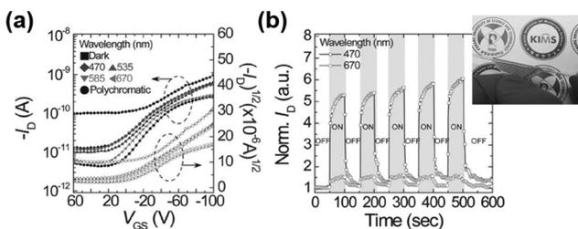
Fig. 3 (a)  $I_D$ - $V_{GS}$  characteristics of PQT-12:PEO nanofiber-based OPTs under light illumination with different wavelengths, and (b) real-time photo-response while the devices were illuminated using a monochromatic light with two different wavelengths. The inset of (b) shows the photograph of a flexible phototransistor array upon bending at a radius of  $\sim 0.75$  mm (reprinted with permission from Lee *et al.*,<sup>49</sup> copyright 2016, Wiley-VCH).
