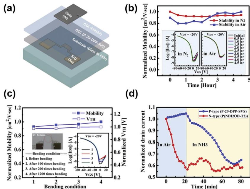
Fig. 17 (a) Schematic representation of a P-29-DPP-SVS-based OFET device. Relationship between the normalized mobility and the effect of (b) air and  $N_2$  ambient, and (c) bending radius of the flexible OFET device. (d) Ammonia-sensing behavior of both p-type P-29-DPP-SVS and n-type P(NDI2OD-T2) materials (reprinted with permission from Ryu *et al.*,<sup>120</sup> copyright 2015, Elsevier B.V.).
