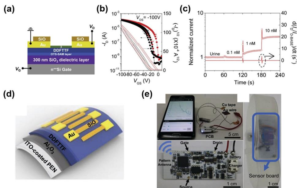
**Fig. 29** (a) Schematic illustration and (b) transfer characteristics of a DDFTF OFET on a silicon substrate, (c) OFET device response toward different concentrations of ATS analytes in urine samples, (d) schematic representation of the DDFTF-based flexible OFET device, (e) photograph demonstrating the integration of the flexible OFET device on the wristband for real-time monitoring application (reprinted with permission from Jang *et al.*,<sup>238</sup> copyright 2017, Elsevier Inc.).
