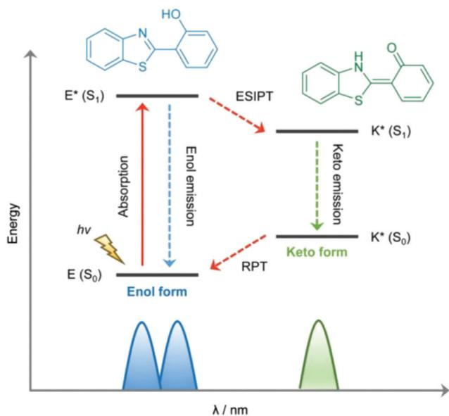
Fig. 5 Mechanistic representation of excited state intramolecular proton transfer. Reproduced from *Chem. Soc. Rev.* 2018, **47**, 8842–8880, with permission from the Royal Society of Chemistry.
