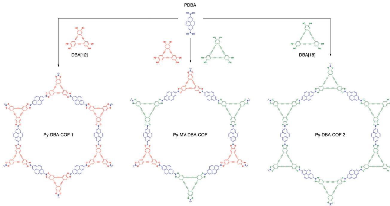
Fig. 11 Synthesis of Py-DBA-COF 1, Py-MV-DBA-COF, and Py-DBA-COF 2.
