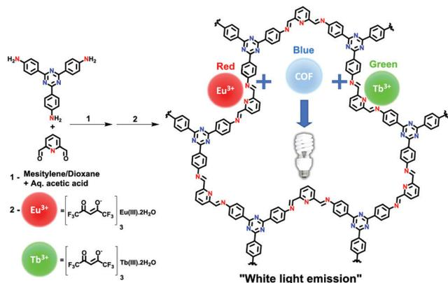
Fig. 33 Synthetic scheme for the formation of TTA-DFP COF and the subsequent grafting of lanthanides. Reprinted with permission from *ACS Appl. Mater. Interfaces*, 2019, **11**, 27343–27352. Copyright 2019 American Chemical Society.
