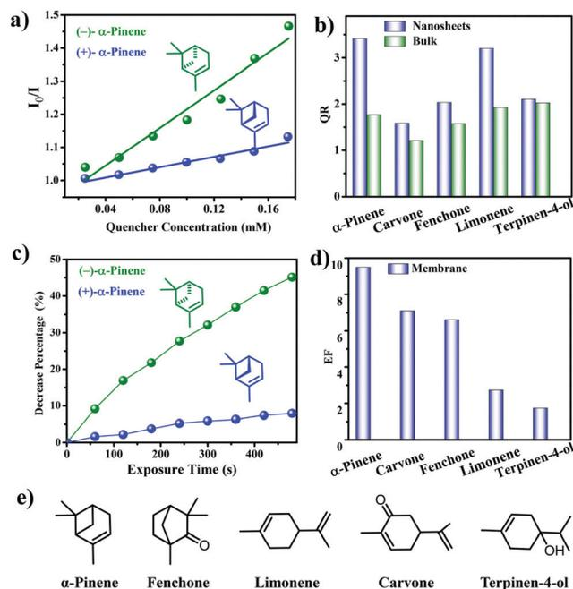
Fig. 23 (a) Stern–Volmer plots of 7-NS in MeCN after titration of  $\alpha$ -pinene. (b) Enantioselective quenching ratios for various terpenes. (c) Decreased fluorescence (%) of 7@PVDF upon introduction of  $\alpha$ -pinene. (d) Enantioselective quenching ratios for various terpene vapors. (e) Structures of terpenes used. Reprinted with permission from *J. Am. Chem. Soc.*, 2019, **141**, 7081–7089. Copyright 2019 American Chemical Society.
