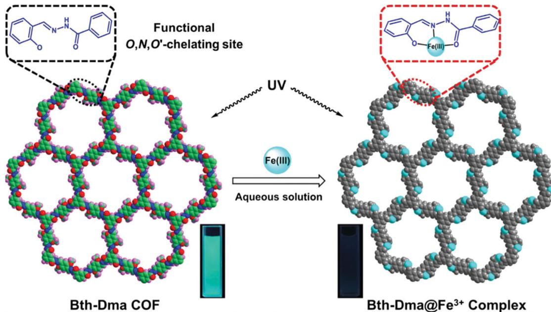
Fig. 21 Structure of Bth-Dma COF with and without the addition of Fe<sup>3+</sup>. Inset photographs show the fluorescence quenching upon the formation of Bth-Dma@Fe<sup>3+</sup> complex. Reprinted with permission from *ACS Appl. Mater. Interfaces*, 2019, **11**, 12830–12837. Copyright 2019 American Chemical Society.
