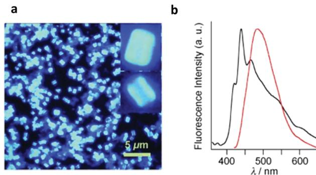
Fig. 10 (a) Fluorescence microscopic image of PPy-COF (the inset depicts an enlarged image of individual cubes). (b) Normalized fluorescence spectra ( $\lambda_{\text{ex}} = 414$  nm, 25 °C) of PDBA (black curve) and PPy-COF (red curve). Adapted with permission from *Angew. Chem., Int. Ed.*, 2009, **48**, 5439–5442.
