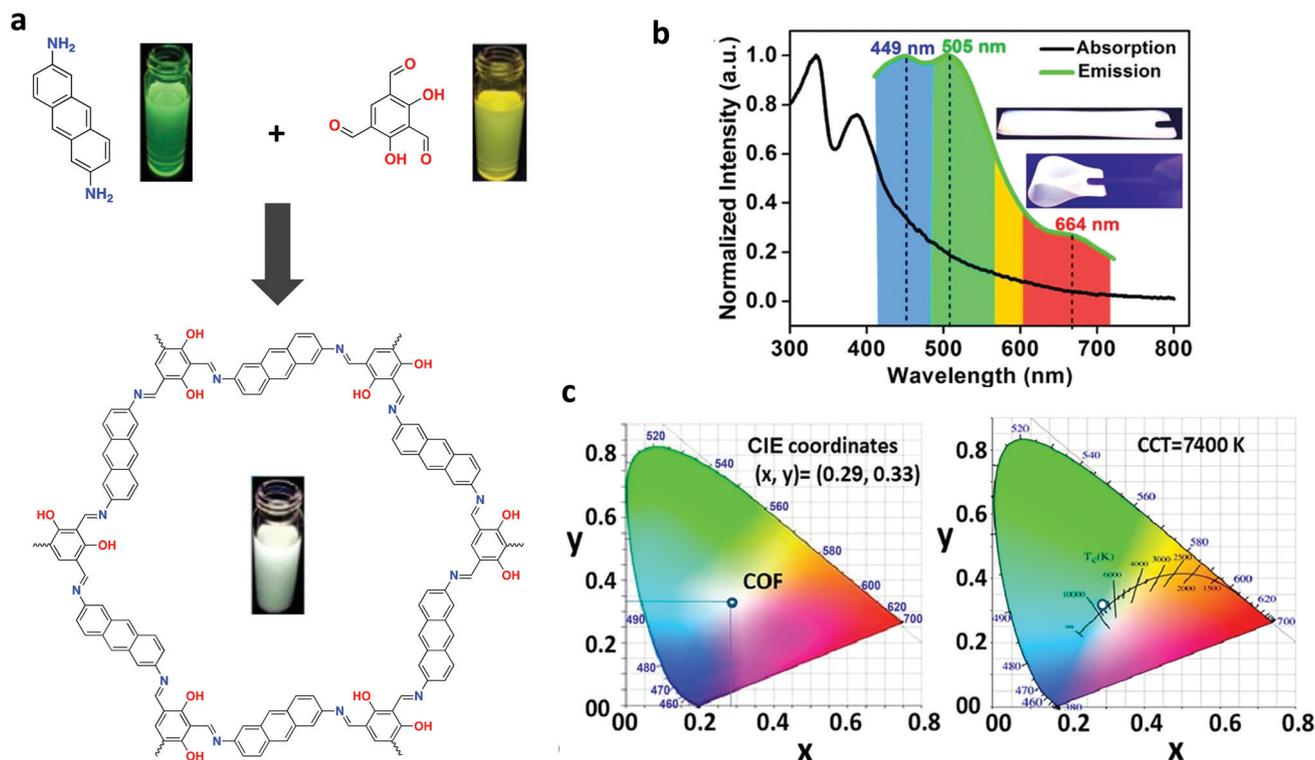
Fig. 34 (a) Synthesis of IISERP-COF7, including photographs of monomers and COF dispersed in NMP under a UV lamp. (b) Solid state absorption and emission spectra of COF@PMMA ( $\lambda_{\text{ex}} = 420 \text{ nm}$ ), with inset photographs of COF@PMMA film under UV irradiation. (c) CIE coordinate and CCT diagram of COF film with a thickness of 2 mm. Adapted with permission from *J. Am. Chem. Soc.*, 2018, **140**, 13367–13374. Copyright 2018 American Chemical Society.
