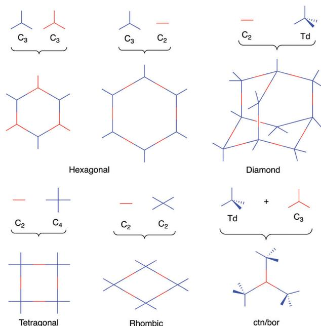
Fig. 1 Sample of topologies accessible through COF synthesis.
