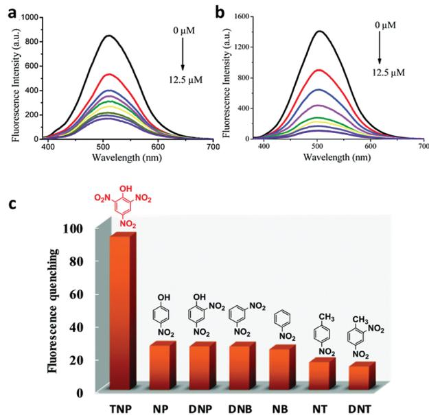
**Fig. 16** Fluorescence spectra ( $\lambda_{\text{ex}} = 370$  nm) of (a) COF-BABD-DB and (b) COF-BABD-BZ dispersed in MeCN with the addition of varying amounts of TNP. (c) Fluorescence quenching (%) of COF-BABD-BZ with different nitroaromatics (12.5  $\mu\text{M}$ ). (d) Photographs of COF-BABD-DB dispersed in MeCN with the addition of various nitroaromatics (4.0  $\mu\text{M}$ ). Adapted from *Chem. Commun.*, 2018, **54**, 2308–2311, with permission from the Royal Society of Chemistry.
