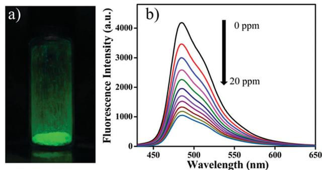
**Fig. 18** (a) Photograph of 3D-Py-COF powder under UV light irradiation. (b) Fluorescence quenching of 3D-Py-COF in DMF upon addition of TNP (0–20 ppm). Reprinted with permission from *J. Am. Chem. Soc.*, 2016, **138**, 3302–3305. Copyright 2016 American Chemical Society.
