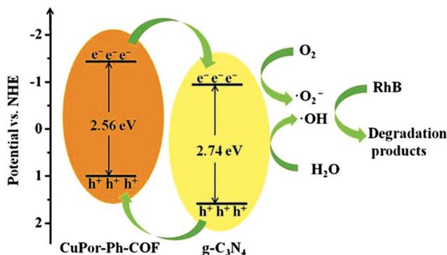
Fig. 31 Proposed mechanism for the photocatalytic degradation of rhodamine B by CuPor-Ph-COF/g-C<sub>3</sub>N<sub>4</sub> hybrid composite. Reproduced from *Dalton Trans.*, 2019, **48**, 14989–14995, with permission from the Royal Society of Chemistry.
