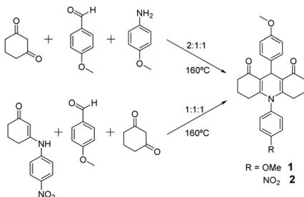
Scheme 1 Synthetic procedure for 1 and 2.
