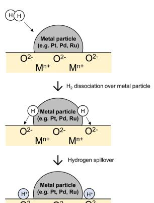
Fig. 1 Schematic images of spillover of H atoms from metal particles to reducible metal oxides.
