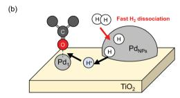
Fig. 2 Schematic image of the ketone/aldehydes hydrogenation over  $Pd_1/TiO_2$  (a) and  $Pd_{1+NPs}/TiO_2$  (b).
