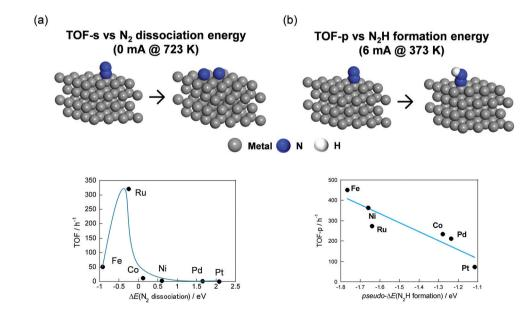
Fig. 15 Illustration of DFT calculation models and relation between TOF-s without the electric field and N2 dissociation energy (a), TOF-p with the electric field, and N2H formation energy (b).
