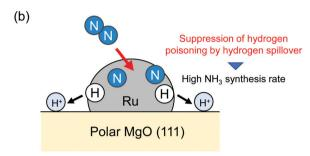
Fig. 6 Hydrogen poisoning suppression by hydrogen spillover.
