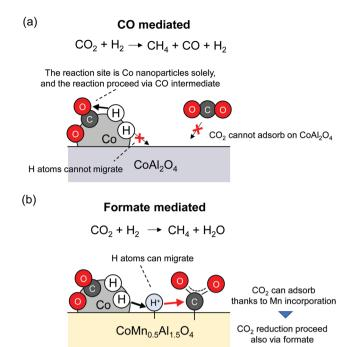
Fig. 5 Change of CO<sub>2</sub> methanation mechanism by addition of Mn.
