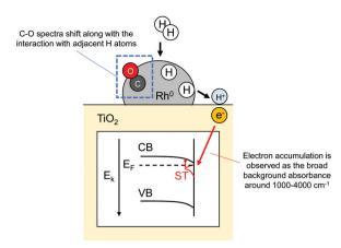
Fig. 7 Illustration of FT-IR measurement for detecting H atoms adsorption over Rh<sup>0</sup> and n-doping into TiO<sub>2</sub>.
