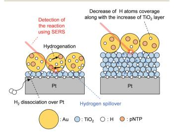
Fig. 9 Schematic image of hydrogen spillover on a Au/TiO $_2$ /Pt sandwich sample.
