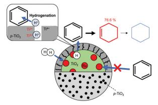
Fig. 4 Selective hydrogenation of benzene over (Ru/TiO<sub>2</sub>)@p-TiO<sub>2</sub>.
