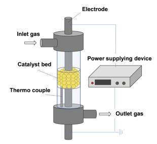
Fig. 12 Schematic image of the apparatus for catalytic reaction in the electric field.
