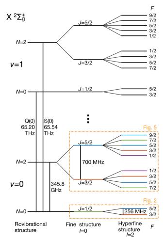
Fig. 1 Partial schematic of the field-free energy levels of  $N_2^+$  in the electronic ground state, X  $^2\Sigma_q^+$  (not to scale). The states are labeled using the Hund's case ( $b_{\beta J}$ ) basis eqn (3). The dotted boxes indicate the level subspaces shown in Fig. 2 and 5 where the relevant Zeeman manifolds are displayed. The color coding of the levels is identical with the one used in these figures
