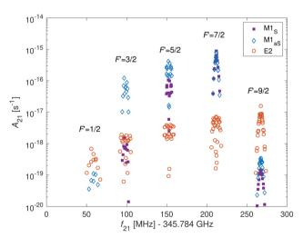
Fig. 9 Einstein A coefficients of hyperfine-Zeeman components of the spin-rotational transition  $|N=0, J=1/2, F=5/2\rangle \rightarrow |N'=2, J'=5/2, F'\rangle$  of the I = 2 nuclear-spin species. Transitions due to M1<sub>S</sub>, M1<sub>aS</sub> and E2 are indicated by purple squares, blue diamonds and red circles. The magnetic field was set to 5 G.
