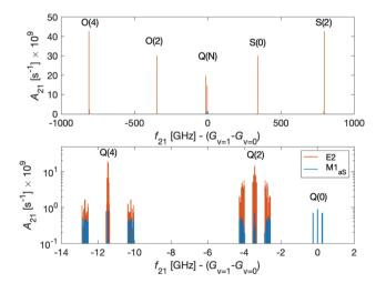
Fig. 10 Einstein A coefficients of E2 (red lines) and  $M1_{aS}$  (blue lines) transitions of the O(N = 2, 4), Q(N = 0, 2, 4) and S(N = 0, 2) branches of the fundamental vibrational transition  $|v = 0, N\rangle \rightarrow |v' = 1, N'\rangle$ . The magnetic field was assumed to be 5 G. The lower panel shows a magnification of the spectrum in the region of the Q branch.
