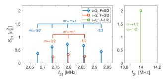
Fig. 3 Strengths,  $S_{21}$ , of M1<sub>S</sub> transitions,  $m \rightarrow m'$ , between Zeeman levels within the hyperfine manifolds of the rovibronic ground state, X  $^2\Sigma_q^+$  (v=0, N=0), of the I=0 (green) and I=2 (blue and red) nuclear-spin species of  $N_2^+$  as a function of transition frequency,  $f_{21}$ . The abscissa indicates the transition frequencies at a magnetic field of 5 G. The color code is the same as in Fig. 2.
