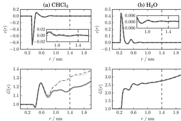
Fig. 9 Dipole-dipole orientation correlation functions (DOCs) and distance-dependent Kirkwood factors  $G(r)$  for  $\text{CHCl}_3$  and  $\text{H}_2\text{O}$ . This figure is analogous to Fig. 4 (see the corresponding caption for more information). Comparison of results with lattice-sum (thick gray), 4–6 RF/AT/SW (dotted) and 0.75 RF/AT/SW (dashed). Straight-cutoff with AT truncation is used for the LJ interactions in all cases.
