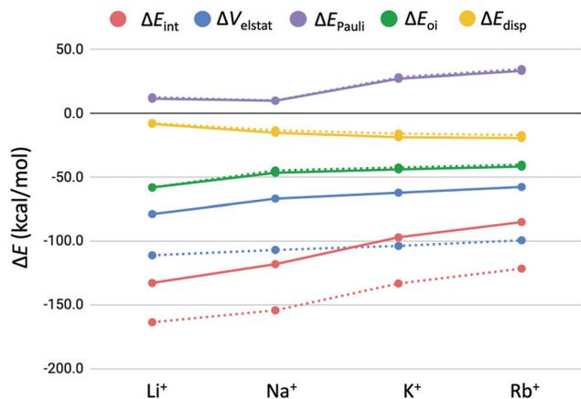
Fig. 6 Energy decomposition of the interaction energy (in kcal mol<sup>-1</sup>) between the alkali metal cations (M<sup>+</sup>) and GQ-[ ] (dashed lines) and GQ-K<sup>+</sup>-[ ] (solid lines).
