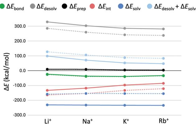
Fig. 5 Partitioning of the bond energy (in kcal mol<sup>-1</sup>) between the alkali metal cations (M<sup>+</sup>) and GQ-[ ] (dashed lines) and GQ-K<sup>+</sup>-[ ] (solid lines).
