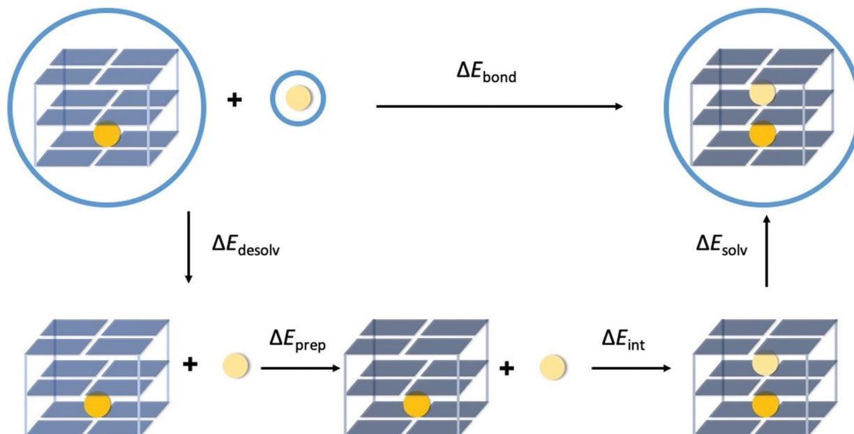
Fig. 3 Partitioning of the bond energy between the second alkali metal cation (light yellow sphere) in the empty cavity of the by  $K^+$  (orange sphere) occupied triple-layer guanine quadruplex structure. The blue circles surrounding the structures indicate that the calculation is performed with COSMO to simulate water.
