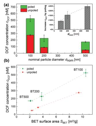
Fig. 4 Pyrocatalytic activity of poled and unpoled BaTiO<sub>3</sub> catalysts with nominal particle sizes of 100, 200 and 500 nm (BT100, BT200, BT500). (a) 2',7'-Dichlorofluorescein (DCF) concentration  $c_{\rm DCF}$  after thermal treatment. Inset plot: Relative increase of  $c_{DCF}$  through poling of BT. (b) Plot of  $c_{DCF}$  as a function of BET surface area  $S_{BET}$ . BET: Brunauer-Emmett-Teller.
