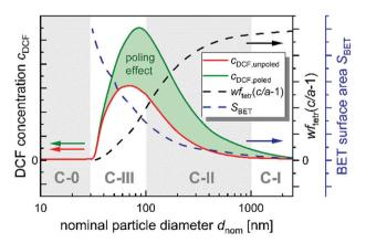
Fig. 5 Hypothetical progression of  $c_{\rm DCF}$ , the product of the tetragonal phase weight fraction wf<sub>tetr</sub> times the tetragonality (c/a-1) and S<sub>BET</sub> as a function of the nominal particle diameter  $d_{\text{nom}}$ . BET: Brunauer-Emmett-Teller.
