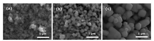
Fig. 2 SEM micrographs of unpoled BaTiO<sub>3</sub> powders with nominal particle sizes of 100, 200 and 500 nm (BT100, BT200, BT500).
