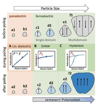
Fig. 6 Schematic representation of the relationships between particle size, polarization, crystal and domain structure (a1)-(f1) before poling and (a2)-(f2) after poling with a sufficiently strong external electric field. Typical progressions of polarization versus electric field (P-E) for (A) paraelectric, (B) ferroelectric single-domain, and (C) ferroelectric multidomain crystals (demonstration only; not to scale)
