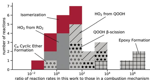
Fig. 12 Histogram of the average ratio of rates calculated in this work and those estimated in the Sarathy mechanism<sup>15</sup> between 500–1000 K, grouped by reaction type.
