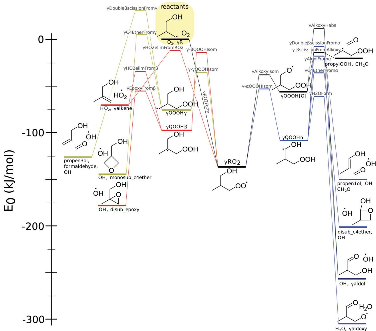
Fig. 9 The potential energy surface for the  $\gamma$ -peroxy radical. Energy includes zero-point energy and atom corrections. Species name and structures appear in black near the structure energy level. Reaction names appear in gray above the transition state energy.
