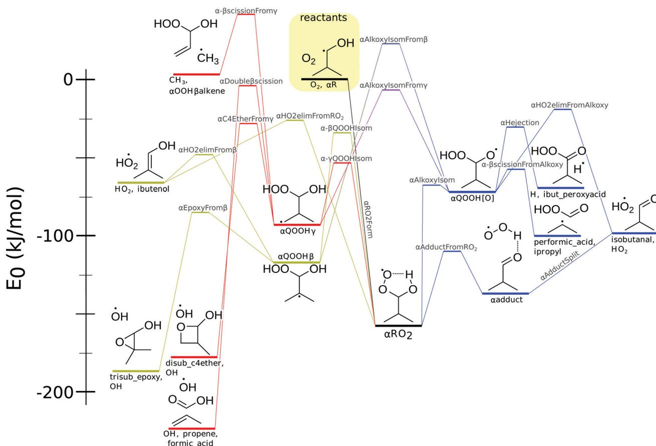
Fig. 3 The potential energy surface for  $\alpha$ -peroxy radical, showing pathways involving  $\alpha$ QOOH (red),  $\alpha$ QOOH (yellow) and  $\alpha$ QOOH[O] (blue). Energy includes zero-point energy and atom corrections.
