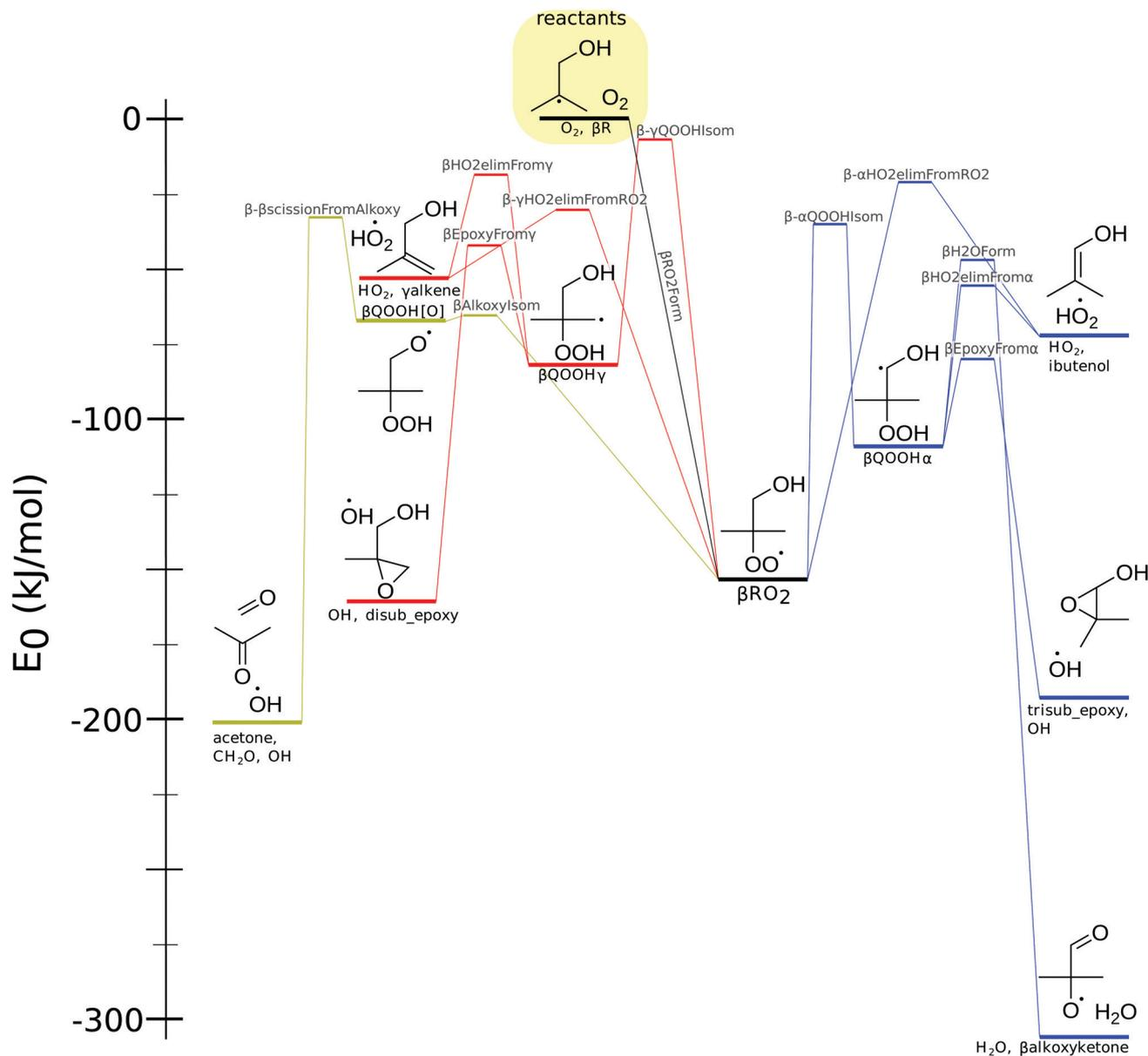
Fig. 6 The potential energy surface for  $\beta$ -peroxy radical, showing pathways involving  $\beta QOOH\gamma$  (red),  $\beta QOOH\alpha$  (blue) and  $\beta QOOHIO$  (yellow). Energy includes zero-point energy and atom corrections.
