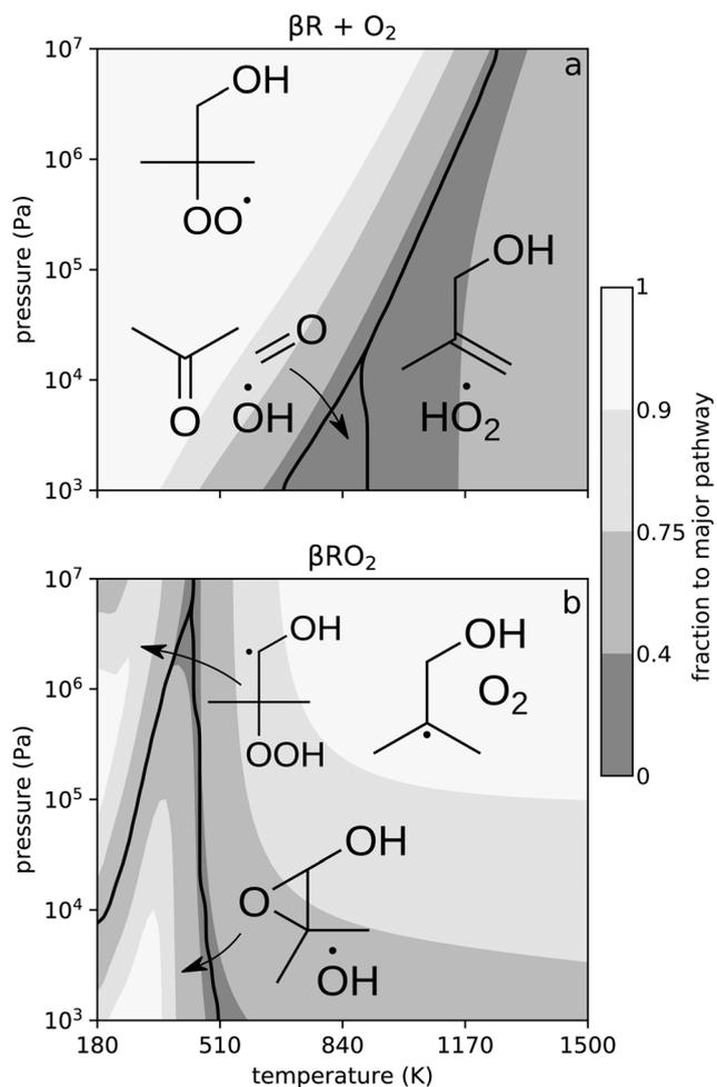
**Fig. 8** Major stabilized products for the reactions of (a)  $\beta\text{R} + \text{O}_2$  and (b)  $\beta\text{RO}_2$  at various temperatures and pressures. Shading indicates the fraction going to the major pathway.
