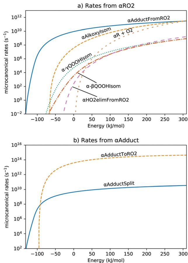
Fig. 4 Microcanonical rates for all the reaction channels coming from (a)  $\alpha\text{RO}_2$  and (b)  $\alpha\text{adduct}$ . The reaction names correspond to those in Fig. 3, with  $\alpha\text{R} + \text{O}_2$  being the reverse of  $\alpha\text{RO}_2\text{Form}$ , and  $\alpha\text{RO}_2\text{Isom}$  being the reverse of  $\alpha\text{AdductFromRO}_2$ . The energy values correspond to those in Fig. 3 and are relative to that of  $\alpha\text{R} + \text{O}_2$ .
