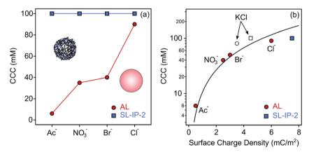
Fig. 3 CCC values of AL (red circles) and SL-IP-2 (blue square) determined in the presence of ILs (a) and CCC versus the charge density data (b). The empty symbols indicate the data measured with KCl. The lines in (a) were added merely to guide the eyes, while in (b), it was calculated using eqn (12).
