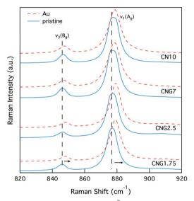
Fig. 8 Raman spectra of select  $MoO_4^{2-}$  vibrational modes ( $\nu_1(A_0)$ 878 cm<sup>-1</sup> and  $\nu_3(B_0)$  848 cm<sup>-1</sup>) in GCs illustrating a spectral shift to higher wavenumbers
