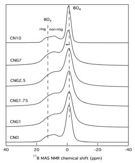
Fig. 4 Mass normalised <sup>11</sup>B MAS NMR spectra for samples with increasing amounts of MoO<sub>3</sub>. The samples with the letter G in the name contain a gadolinium dopant, which can account for the observed peak broadening in these samples.
