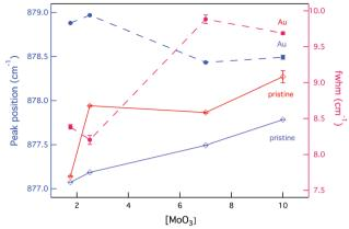
Fig. 9 Changes to the position and broadening of the Raman vibrational band  $\nu_1(A_0)$  as a function of composition and external radiation.
