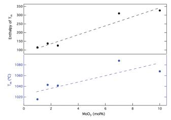
Fig. 3 Melting temperature  $(T_M)$  of CaMoO<sub>4</sub> and the enthalpy of transition for soda lime borosilicate with increasing amounts of MoO<sub>3</sub>.
