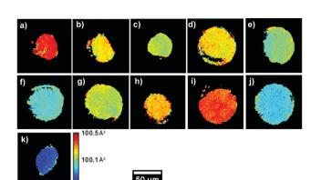
Fig. 3 Unit volume V obtained from the refinement of the coarse scans for (a) the uncycled electrode, (b) 42–25, (c) 42–50, (d) 42–75, (e) 42–100–1, (f) 42–100–2, (g) 47–25, (h) 47–50, (i) 47–75, (j) 47–100–1 and (k) 47–100–2.
