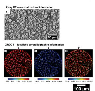
Fig. 4 (a) Absorption micro X-ray CT slice in the through-plane direction for the uncycled NMC electrode. ROI XRD-CT maps for (b) a, (c) c lattice parameters and the (d) unit volume V.
