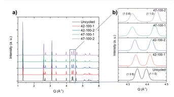
Fig. 2 (a) Diffraction pattern for the uncycled electrodes and those cycled to 100 cycles. Intensity in arbitrary units (a.u.). (b) Expanded view of the (108) and (110) reflections. Diffraction measurements taken with a beam energy of 50 keV, corresponding to a wavelength of 0.2480 Å.
