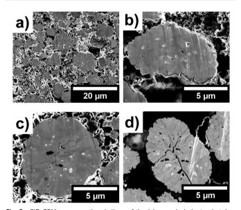
Fig. 9 FIB-SEM cross-sectional slices of the (a) uncycled electrode taken at  $2k\times$ , (b) uncycled particle taken at  $8k\times$ , and particles extracted from (c) 42-100-1 taken at  $8k \times$  and (d) 47-100-1 taken at  $6.5k \times$ .
