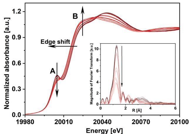
Fig. 2 *In situ* Mo K-edge XANES spectra and corresponding  $k^3$ -weighted Fourier transformed EXAFS spectra (inset) of the FeMo catalyst during TPR under 5% MeOH/He. Arrows point towards increasing temperature.
