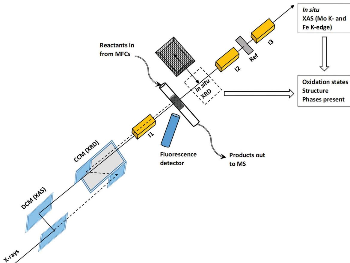
Fig. 1 Schematic setup for *in situ* XAS/XRD experiments performed at the unique setup at SNBL beamline BM31, ESRF. Double crystal monochromator (DCM), channel-cut monochromator (CCM), ionization chambers (I1, I2 and I3), reference foil (Ref), mass flow controllers (MFCs) and mass spectrometer (MS).
