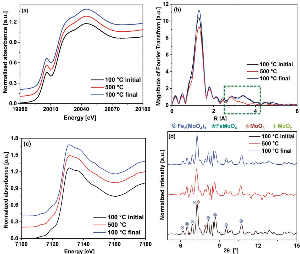
Fig. 8 Comparison of the initial state of the catalyst measured at 100 °C, the state at 500 °C after TPO and the final state after cool-down to 100 °C under 10% O<sub>2</sub>/He: (a) Mo K-edge XANES (b) corresponding  $k^3$ -weighted FT EXAFS spectra with marked region 2.5–4.0 Å. (c) Fe K-edge XANES and (d) XRD patterns with the assignment of phases.
