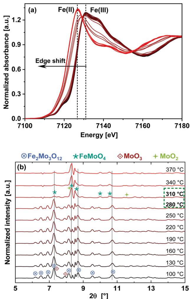
Fig. 4 (a) *In situ* Fe K-edge XANES spectra for the catalyst during heating in 5% MeOH/He (TPR). Dashed lines indicate the energy positions of the white line peak for oxidized and reduced Fe phases. The arrow points towards increasing temperature. (b) *In situ* XRD at 0.4934 Å (25.13 keV) during TPR in 5% MeOH/He. Phase transition to FeMoO<sub>4</sub> can be observed by the increasing intensity of the reflections at 8.32 and 8.50°.
