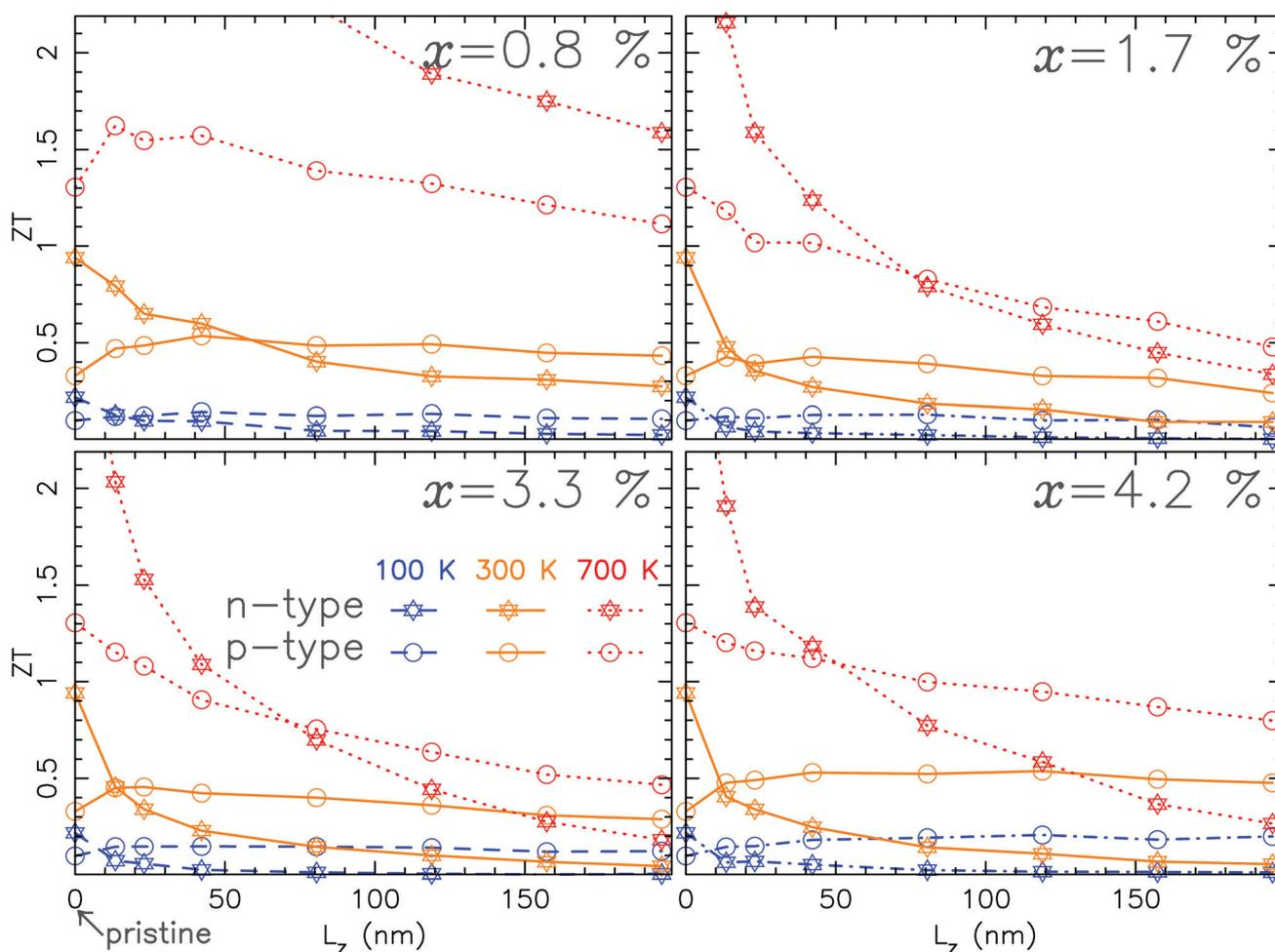
Fig. 6 Figure of merit as a function of the length of the system for 4 different sulfur vacancy concentrations and 3 different temperatures. Note that the values at  $L_z = 0$  correspond to the pristine case.
