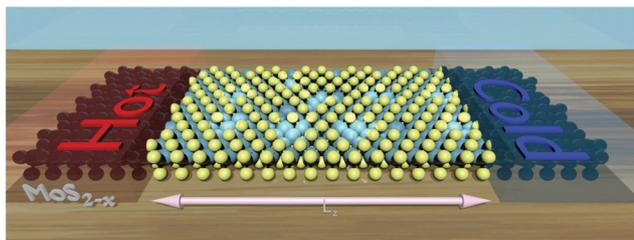
Fig. 1 Artwork of a MoS<sub>2</sub> monolayer within the Landauer formalism. The leads correspond to pristine MoS<sub>2</sub> and the device (between the two leads) corresponds to MoS<sub>2</sub> with randomly located sulfur vacancies.
