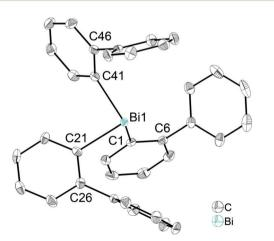
Fig. 1 Thermal ellipsoid model of  $(2-PhC_6H_4)_3Bi$  (1) at 50% probability level. Hydrogen atoms are omitted for clarity. Selected bond lengths [Å]: Bi1-C1 2.258(3), Bi1-C21 2.267(3), Bi1-C41 2.257(4), Bi1···Ph<sub>centroid(I)</sub> 4.06, Bi1···Ph<sub>centroid(II)</sub> 4.04, Bi1···Ph<sub>centroid(III)</sub> 3.99. Selected bond angles [°]: C1-Bi1-C21 95.28(12), C1-Bi1-C41 96.04(12), C21-Bi1-C41 92.33(12), Bi1-C1-C6 118.1(2), Bi1-C21-C26 118.0(3), Bi1-C41-C46 117.0(2)
