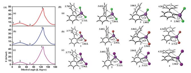
level of theory (1 and 3 (2 and 4)) denotes the local minima (maxima) of the respective compound). (B) Selected conformers of (2-PhC<sub>6</sub>H<sub>4</sub>)BiX<sub>2</sub> taken from PES; (a) X = Cl, (b) X = Br, (c) X = I. Respective dihedral angle, shortest hydrogen bond distance between the nearest hydrogen (H) atom and halogen (X), center-to-center distance between bismuth atoms and phenyl moieties are shown in each geometry. For details on the dihedral definition see ESI.†
