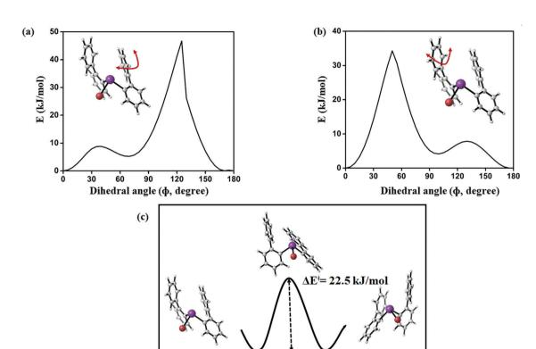
Fig. 19 (a and b) Computed potential energy surface of aryl ring rotation for  $(2-PhC_6H_4)_2BiBr$  (3) and (c) calculated barrier between equivalent conformations of 3 (PBE-D3/def2-TZVP) level of theory.
