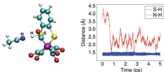
Fig. 6 (a) Snapshot of  $\mathbf{1SH}^-$  in acetonitrile solution. (b) Distances between sulfur and the proton (blue) and between nitrogen and the proton (red) during the simulation, showing the weak hydrogen bond formed between the solvent and the sulfur.
