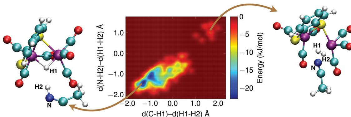
Fig. 11 Free energy surface of the  $H_2$  formation reaction via direct protonation of the bridging hydride of the  $1H^{2-}$  intermediate from the solvent. A metadynamics simulation snapshot of the reactant state is shown on the left, and of the product state on the right. See main text for further details.
