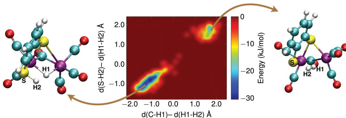
Fig. 13 Free energy surface of the  $\text{H}_2$  formation reaction via internal proton transfer from the sulfur to the bridging hydride. A metadynamics simulation snapshot of the reactant state is shown on the left, and of the product state on the right. See main text for details.
