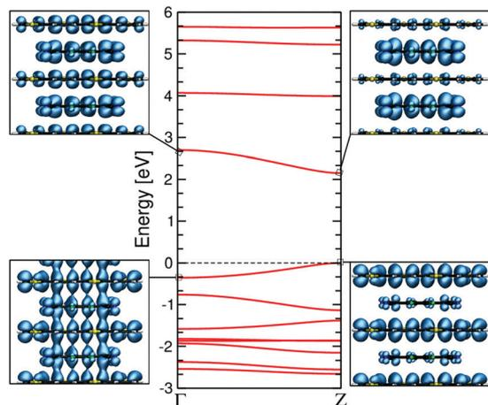
Fig. 5 Quasi-particle band structure of the periodic 4T-F4TCNQ stack. The square modulus of the highest-occupied and lowest-unoccupied Kohn–Sham states at  $\Gamma$  (left) and at  $Z$  (right) is shown.
