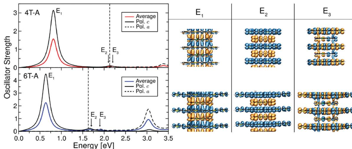
Fig. 8 (left) Optical absorption spectra of periodic 4T- and 6T-F4TCNQ stacks. Black solid (dashed) lines indicate the absorption with polarization along the *c* (*a*) axis in the unit cell (see the reference system at the bottom of Fig. 1), while in color, we depict the average between the two. Dashed bars mark the energy of the QP gaps. (right) Transition densities of the excited states highlighted in the spectra.
