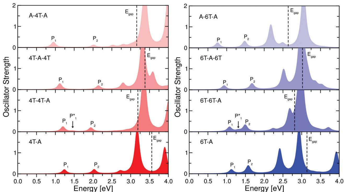
Fig. 6 Optical absorption spectra of isolated dimer and trimer structures with 4T (left) and 6T (right) as donor species. In each spectrum, the energy of the QP gap ( $E_{\text{gap}}$ ) is marked by a vertical dashed line. A broadening of 0.1 eV is applied to all spectra to mimic the excitation lifetime.
