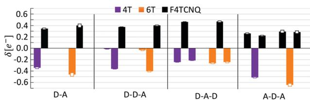
Fig. 2 Charge transfer in the ground state quantified through the Bader analysis of the partial charges on the donor(s) to the acceptor(s) in the CTCs analyzed in this work. The empty portions of the bar indicate the error in the numerical integration of the total charge density, performed on a finite spatial mesh.
