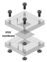
Fig. 2 3D sketch of a microfluidic extraction circuit card with: PTFE membranes; four tightening bolts for mechanical stability; PMMA blocks milled with microfluidic serpentine channels; input/output stainless steel tubes. The volume of each channel within the phase contact area is  $35.7 \,\mu$ L. Reprinted from ref. 34, Copyright 2019, with permission from Elsevier.
