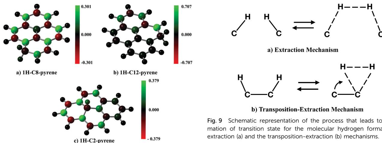
Fig. 9 Schematic representation of the process that leads to the formation of transition state for the molecular hydrogen formation: the extraction (a) and the transposition-extraction (b) mechanisms.
