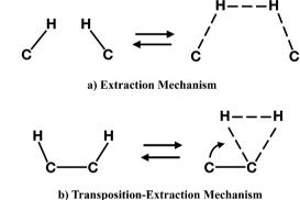
Fig. 9 Schematic representation of the process that leads to the formation of transition state for the molecular hydrogen formation: the extraction (a) and the transposition-extraction (b) mechanisms.
