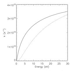
Fig. 11 Comparison between reaction rates for the forward reaction toward SW-pyrene (solid line) and for the reverse reaction toward pristine pyrene (dashed line) as a function of internal energies. Rates were calculated using the RRKM formalism<sup>51,55</sup> starting from the energies and vibrational analysis performed in this paper at the M06-2X/pcseq-1 level.
