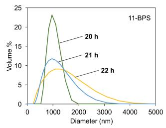
Fig. 5 Particle distribution measured with DLS in dispersions of milled Fe:LiNbO<sub>3</sub> particles, milled in the presence of **11-BPS** for 20, 21, and 22 h.
