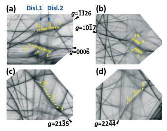
Fig. 14 LACBED pattern as observed from the dislocations under a 2C-M-pit with the  $\langle 11\bar{2}0 \rangle$  separation, which are the same as shown in Fig. 13. Laue reflection lines using five different g vectors are shown in (a)-(d).
