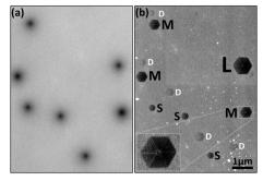
Fig. 4 (a) Panchromatic CL image and (b) secondary electron image taken from the same sample area containing representative etch pits from each size level. L: large; M: middle; S: small; D: dent. The inset in (b) shows an enlarged image of an M-pit with double pit cores (a 2C-M-pit).
