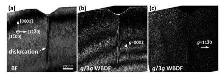
Fig. 11 TEM images of (a) BF, (b) g/3g WBDF with g = 0002, and (c) g/3g WBDF with  $g = 11\bar{2}0$  as observed from a typical "bright" 1C-M-pit with  $I_c = 43.7$  and  $I_d = 225.1$  nm. The results indicate that it is a 1c TSD.
