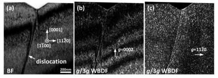
Fig. 12 TEM images of (a) BF, (b) g/3g WBDF with g=0002, and (c) g/3g WBDF with  $g=11\bar{2}0$  as observed from a typical "dark" 1C-M-pit with  $I_c=20.7$  and  $L_d=231.3$  nm. The results indicate that it is an a+c TMD.
