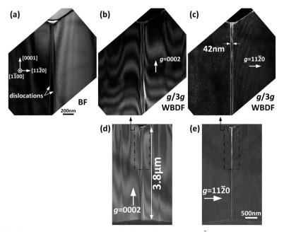
Fig. 13 TEM images of (a) BF, (b) g/3g WBDF with g=0002, and (c) g/3g WBDF with  $g=11\bar{2}0$  as observed from a pair of dislocations under a 2C-M-pit with the  $\langle 11\bar{2}0 \rangle$  separation. (d) and (e) show low-magnification images showing the entire  $\langle 0001 \rangle$  thickness of the TEM foil. The results show that both dislocations are TMDs. The scale bar for (a)–(c) is 200 nm and that for (d) and (e) is 500 nm.
