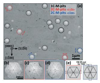
Fig. 10 (a) SEM image of an area containing several types of M-pits. Enlarged images of representative M-pits (marked with solid circles) with a (b) single-core, (c) double-core with a  $\langle 11\bar{2}0 \rangle$  separation, (d) double-core with a  $\langle 1\bar{1}00 \rangle$  separation, and (e) schematics of the 2C-Mpits and the directions of their FIB lift-out. The arrows indicate the direction of separation. The scale bar for (a) is 1 µm and that for (b), (c), and (d) is 200 nm.
