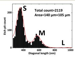
Fig. 7 A histogram showing the pit count as a function of the pit size measured from the diagonal length along the  $\langle 11\bar{2}0\rangle$  direction.
