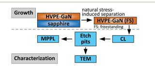
**Fig. 1** A flowchart of the growth and characterization processes. HVPE: hydride vapor phase epitaxy; CL: cathodoluminescence; TEM: transmission electron microscopy; and MPPL: multi-photon excitation photoluminescence.
