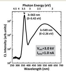
Fig. 2 A typical CL spectrum taken at an accelerating voltage ( $V_{acc}$ ) of 3.0 kV with a probe current ( $I_{ems}$ ) of approximately 1.0 nA.
