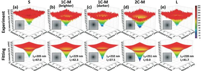
Fig. 5 Observation (upper row) and fitting (lower row) results for representative dark spots corresponding to (a) S-pit, (b) 1C-M-pit with a brighter contrast, (c) 1C-M-pit with a darker contrast, (d) 2C-M-pit, and (e) L-pit.  $L_d$  is the carrier diffusion length, and  $I_c$  is the CL intensity at the TD core.
