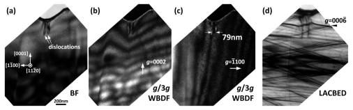
Fig. 15 TEM images of (a) BF, (b) g/3g WBDF with g = 0002, and (c) g/3g WBDF with g = 1100 as observed from a pair of dislocations under a 2C-M-pit with the  $\langle 1\bar{1}00 \rangle$  separation. (d) The LACBED pattern obtained for  $g=000\bar{6}$ . The results show that both dislocations are TMDs. The scale bar for (a)-(c) is 200 nm.
