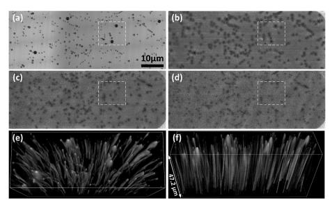
Fig. 18 (a) Etch pit image, and MPPL images taken from the same area at (b) Z = 0, (c)  $Z = 23.6 \mu m$ , and (d)  $Z = 47.2 \mu m$ . (e) and (f) show the 3D reconstructed dislocation images. The dislocation contrast is inverted for a better view.
