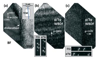
Fig. 8 TEM images of the (a) bright-field (BF), (b) g/3g weak-beam dark-field (WBDF) with g = 0002, and (c) g/3g WBDF with  $g = 11\overline{2}0$ . Selected area diffraction patterns (SADPs) for the WBDF are shown. The inset in (a) shows a schematic drawing showing the lift-out position with respect to the etch pit.
