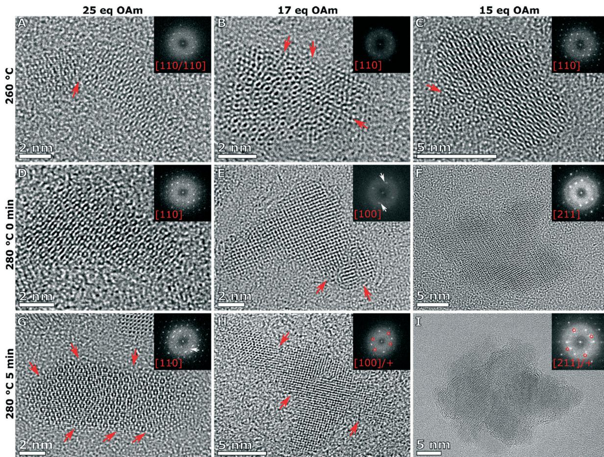
Fig. 7 HRTEM images of particles formed with 25 eq. OAm (A, D and G), 17 eq. OAm (B, E and H) and 15 eq. OAm (C, F and I) taken from different stages in the reaction at 260 °C, 280 °C at 0 min and at 5 min respectively. The red arrows point defects in the structure, white arrows indicating streaking or slight misalignments in the FFTs, and the red circles in the FFTs correspond to additional reflections coming from mis-oriented grains.
