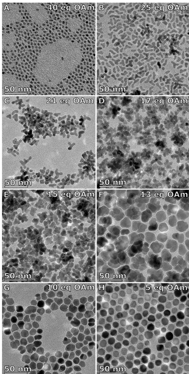
Fig. 2 TEM images of IONPs made with a constant nitrogen purge with A) 40 eq., B) 25 eq., C) 21 eq., D) 17 eq., E) 15 eq., F) 13 eq., G) 10 eq., and H) 5 eq. OAm to the metal precursor  $[\text{Fe}(\text{acac})_3]$ .
