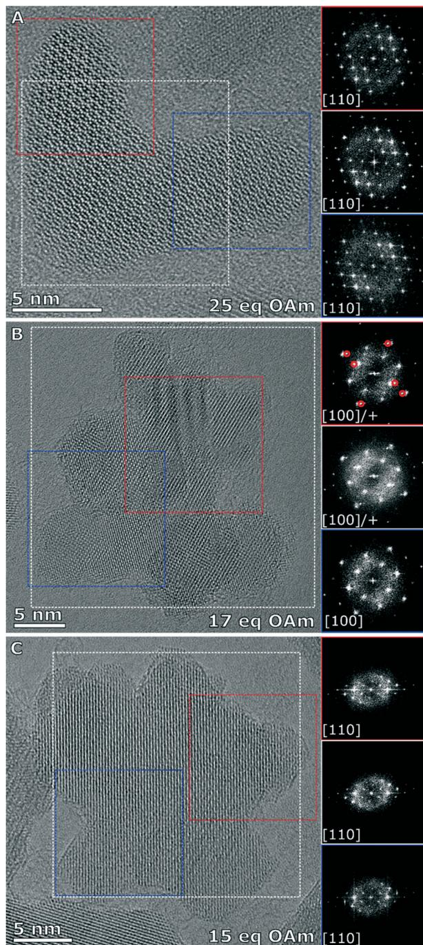
**Fig. 5** High resolution images of the IONPs synthesized with a nitrogen purge and A) 25 eq. OAm (branched), B) 17 eq. OAm (multiply branched) and C) 15 eq. OAm (multiply branched). Each particle has the FFT of the full particle in the white box, and the FFT's of two different regions of the particle indicated by the red and blue boxes respectively.
